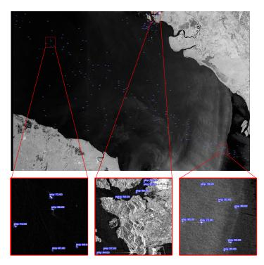
Figure 12. Detection visualization results of the proposed method in a large-scene SAR image.
