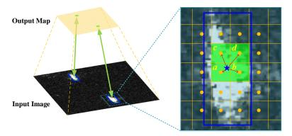
**Figure 8.** An illustration of center-based uniform matching. The orange point and blue star represent grid center and target center, respectively. Additionally, green squares are the assigned positive grids.
