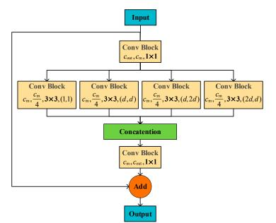
Finally, we add the input feature to the processed feature by adding a residual connection, resulting in an output feature map with multiple receptive fields.
