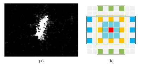
Figure 6. (a) Ship target in SAR image. (b) An illustration of the receptive field of RADC block.
