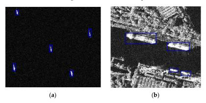
**Figure 1.** Examples of SAR ship targets in [36]. Blue rectangles represent the bounding box of ship targets. (**a**) Small ships in offshore areas. (**b**) Ships in complex inshore backgrounds.
