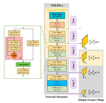
Figure 4. Structure of the CSPDarknet.
