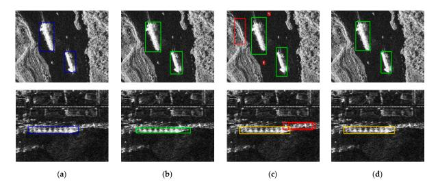
**Figure 10.** Effect of the proposed method. (a) Ground truth. (b) Detection results of YOLOX-s. (c) Detection results of C3. (d) Detection results of the proposed method.
