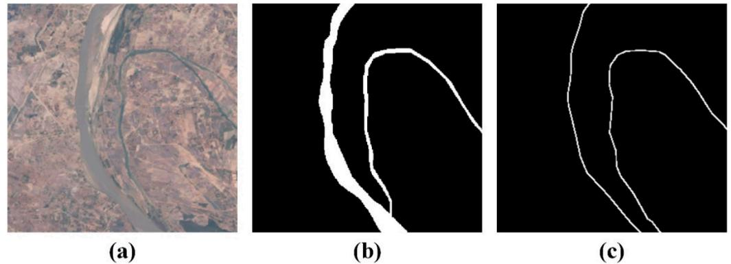
**Figure 1.** (a) Sample patch from very high-resolution Landsat 8 image patch, (b) the pixel-level ground-truth labels, and (c) OSM-based sparse scribbled annotations.
