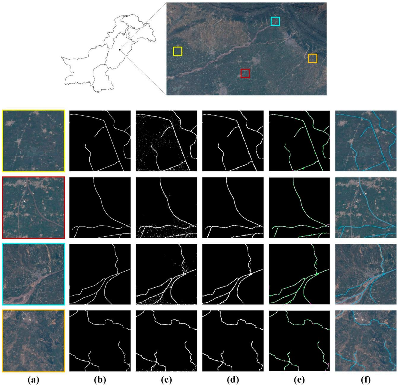
**Figure 7.** Qualitative water channel segmentation results: (a) raw input patches, (b) ground-truth pixels, (c) AUnet segmented labels containing noisy and stray pixels, (d) postprocessed images to remove noisy pixels, and (e) overlapped ground-truth and postprocessed pixels. Magenta depicts the undersegmented (false negative) pixels, and green indicates the oversegmented (false positive) pixels, (f) extracted and overlaid water channels on (a).
