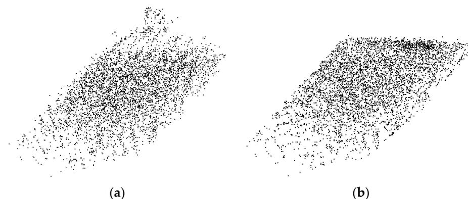
**Figure 9.** Comparison of the original planar point cloud and the projected point cloud. (a) The original planar point cloud. (b) The projected planar point cloud.
