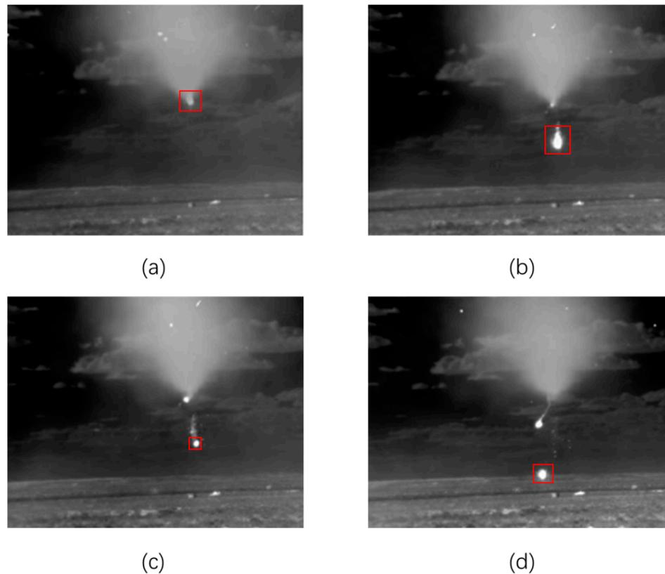
**Figure 1.** Continuous frames of infrared point target abnormal events. (a) The normal flight state of the target. (b) The target is separated, and the debris is separated from the main body. (c,d) Debris and the main target body move together [2].
