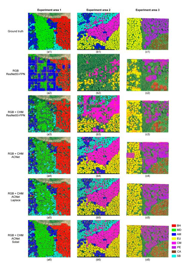
**Figure 7.** The results of individual tree species identification for three experimental areas by different experiment schemes. Different experiment schemes are shown on the left of the figure. (**a**–**c**) Experimental areas 1, 2, and 3, respectively.
