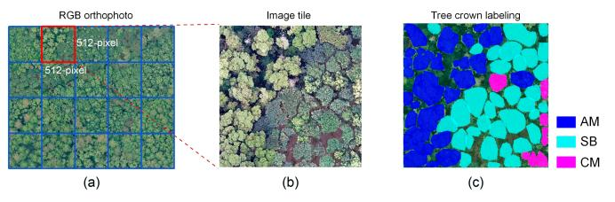
**Figure 2.** Schematic diagram of sample labeling for individual tree species identification. (a) RGB orthophotos. (b)  $512 \times 512$ -pixel image tile. (c) Tree crown labeling results.
