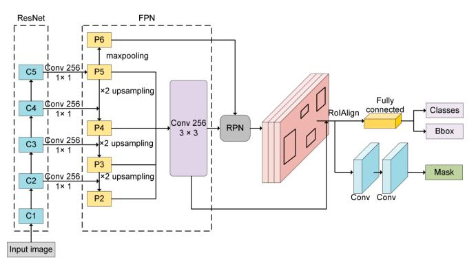
Figure 3. The framework of Mask R-CNN instance segmentation model.
