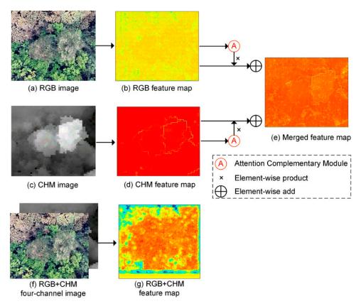
**Figure 10.** Feature map extracted by ACNet (**a**–**e**) and ResNet50-FPN (**f**,**g**). (**b**,**d**,**e**) Feature map extracted from the RGB branch, CHM branch, and fusion branch of ACNet, respectively. (**g**) Feature map extracted by ResNet50-FPN.
