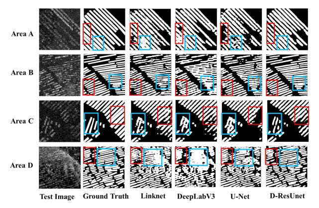
**Figure 6.** Resulting maps of four models in four randomly selected test areas. Black pixels represent the ocean background and white pixels represent the extracted FRA areas. Red rectangles are areas where the FRA area is easily missed, and blue rectangles are areas where the FRA extraction result is prone to adhesions.
