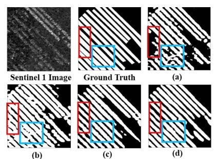
Meanwhile, the resulting maps show that the narrower end of adjacent floating rafts is prone to stick together.
