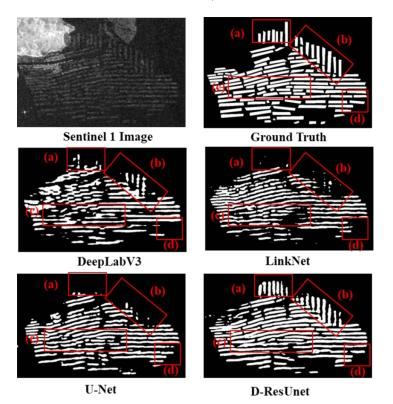
**Figure 8.** Resulting maps of the application experiment. Black pixels represent the seawater and white pixels represent the extracted FRA areas. Red rectangles (a–d) are areas where the FRA area is easily missed.
