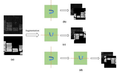
Figure 4. Data augmentation: (a) raw data; (b) horizontal flip; (c) vertical flip; (d) diagonal mirroring.
