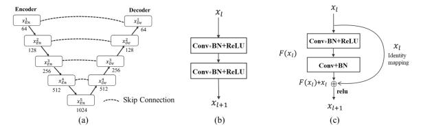
Figure 1. (a) The structure of the U-Net model; (b) Plain neural unit in U-Net; (c) Residual unit.
