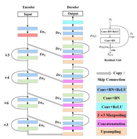
Figure 2. The structure of the proposed D-ResUnet model.
