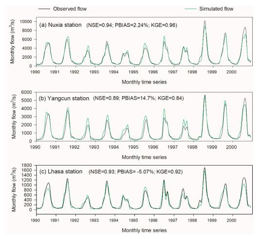
Figure 9. Monthly flow simulation at (a) Nuxia, (b) Yangcun, and (c) Lhasa hydrological stations during calibration period (1990–2000).
