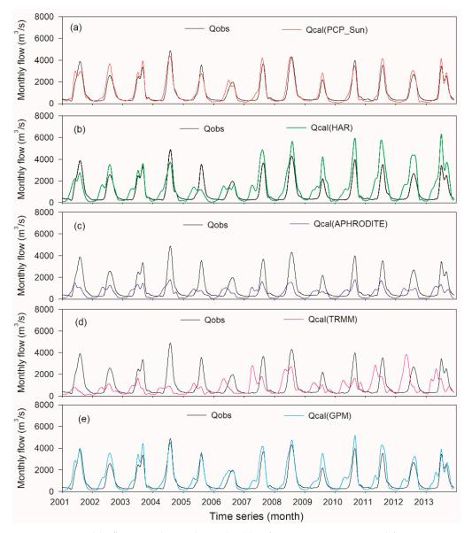
**Figure 11.** Monthly flow simulation driven by (**a**) reference precipitation and four precipitation datasets: (**b**) HAR, (**c**) APHRODITE, (**d**) TRMM and (**e**) GPM, at Yangcun hydrological station during years 2001–2013.
