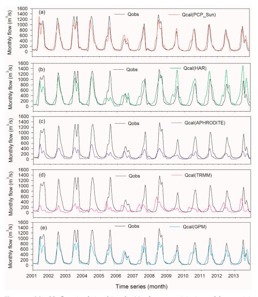
**Figure 12.** Monthly flow simulation driven by (**a**) reference precipitation and four precipitation datasets: (**b**) HAR, (**c**) APHRODITE, (**d**) TRMM and (**e**) GPM, at Lhasa hydrological station during years 2001–2013.
