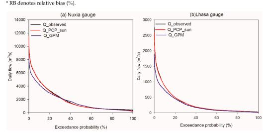
**Figure 13.** Flow duration curves of the observed and simulated daily discharge at (**a**) Nuxia and (**b**) Lhasa hydrological stations.
