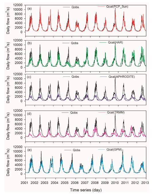
**Figure 7.** Daily flow simulation driven by (**a**) reference precipitationand four precipitation datasets: (**b**) HAR, (**c**) APHRODITE, (**d**) TRMM and (**e**) GPM, at Nuxia hydrological station during years 2001–2013. Qobs represents the observed streamflow. Qcal(PCP\_Sun), Qcal(HAR), Qcal(APHRODITE), Qcal(TRMM) and Qcal(GPM) represent the calculated streamflow using the corresponding individual precipitation dataset.
