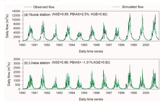
**Figure 6.** Daily flow simulation at Nuxia (**a**) and Lhasa hydrological stations (**b**) during the calibration period (1990–2000).
