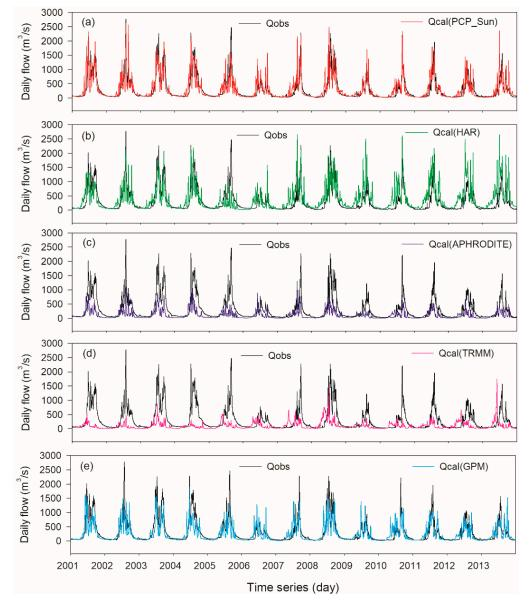
**Figure 8.** Daily flow simulation driven by (**a**) reference precipitation and four precipitation datasets: (**b**) HAR, (**c**) APHRODITE, (**d**) TRMM and (**e**) GPM, at Lhasa hydrological station during years 2001–2013.
