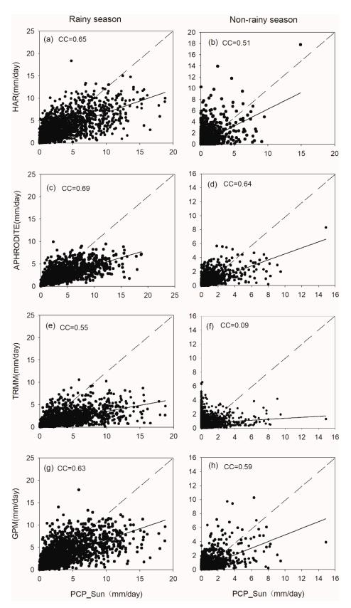
**Figure 5.** Scatterplots of daily basin-wide precipitation between gridded precipitation and reference precipitation during rainy season ((**a**) HAR, (**c**) APHRODITE, (**e**) TRMM, (**g**) GPM), and non-rainy season ((**b**) HAR, (**d**) APHRODITE, (**f**) TRMM, (**h**) GPM). The solid line shows the linear least-squares result, and the diagonal dash line shows the 1:1 line.
