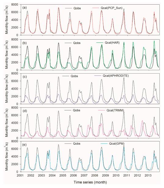
**Figure 10.** Monthly flow simulation driven by (**a**) reference precipitation and four precipitation datasets: (**b**) HAR, (**c**) APHRODITE, (**d**) TRMM and (**e**) GPM, at Nuxia hydrological station during years 2001–2013.
