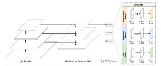
**Figure 7.** GPS-RetinaNet. Similar to RetinaNet [21], this architecture uses a FPN [17] backbone on top of a ResNet [33] model (**a**) to create a convolutional feature pyramid (**b**). Then, we attach three subnetworks (**c**); one for classification, one for box regression, and one for GPS/depth regression.
