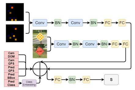
**Figure 9.** The architecture of the similarity network. The network uses two siamese sub-networks and then concatenates all the resulting features. The remaining features are sent through two more fully connected layers before predicting the similarity score.
