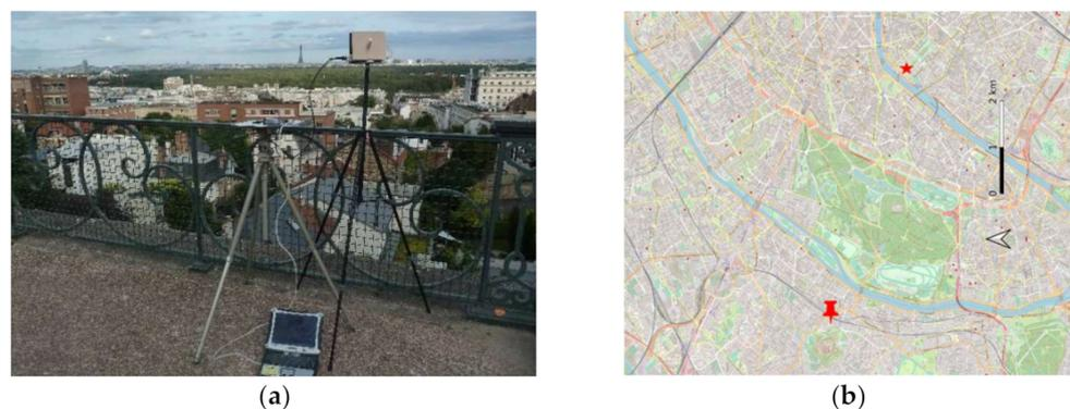
**Figure 14.** (a) Setup of the experiment conducted in Paris, France, at the Mont Valerien location and (b) the aerial picture of the imaging scene, where the experiment site is indicated by the red nail.
