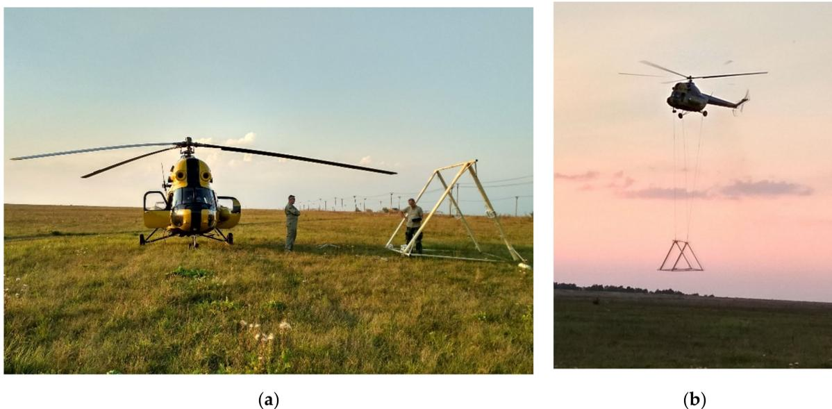
**Figure 1.** Airborne GPR on the landing field (a) and in flight (b).
