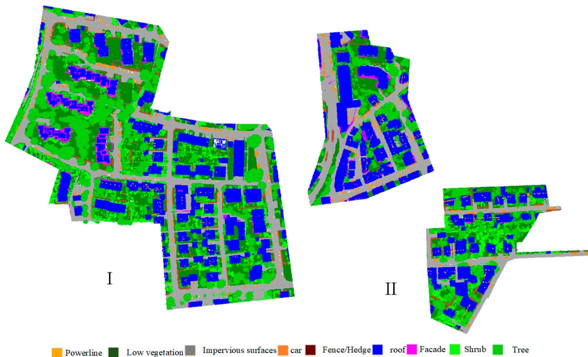
**Figure 4.** Scene I show the data for training and validation. Scene II is the test set. The following nine classes are discerned: power line, low vegetation, impervious surfaces, car, fence/hedge, roof, façade, shrub and tree.
