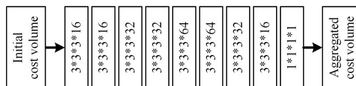
**Figure 9.** The plain module for cost aggregation in DSM-Net-v3. In this variant, the 4D volume output by the eighth convolution layer at the low scale is up-sampled and added to the initial cost volume at the high scale. Each convolution layer is followed by a batch normalization layer and a leaky ReLU activation layer ( $\alpha = 0.3$ ), except for the last two layers.
