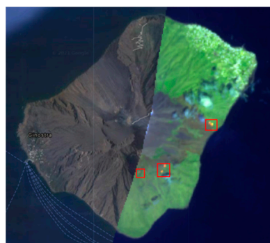
Figure 9. Fires detected at Stromboli after the 3 July 2019 paroxysm. False Color image made by B12-B11-B4 bands from Sentinel-2 MSI image acquired on 4 July 2019 at 09:49 UTC.
