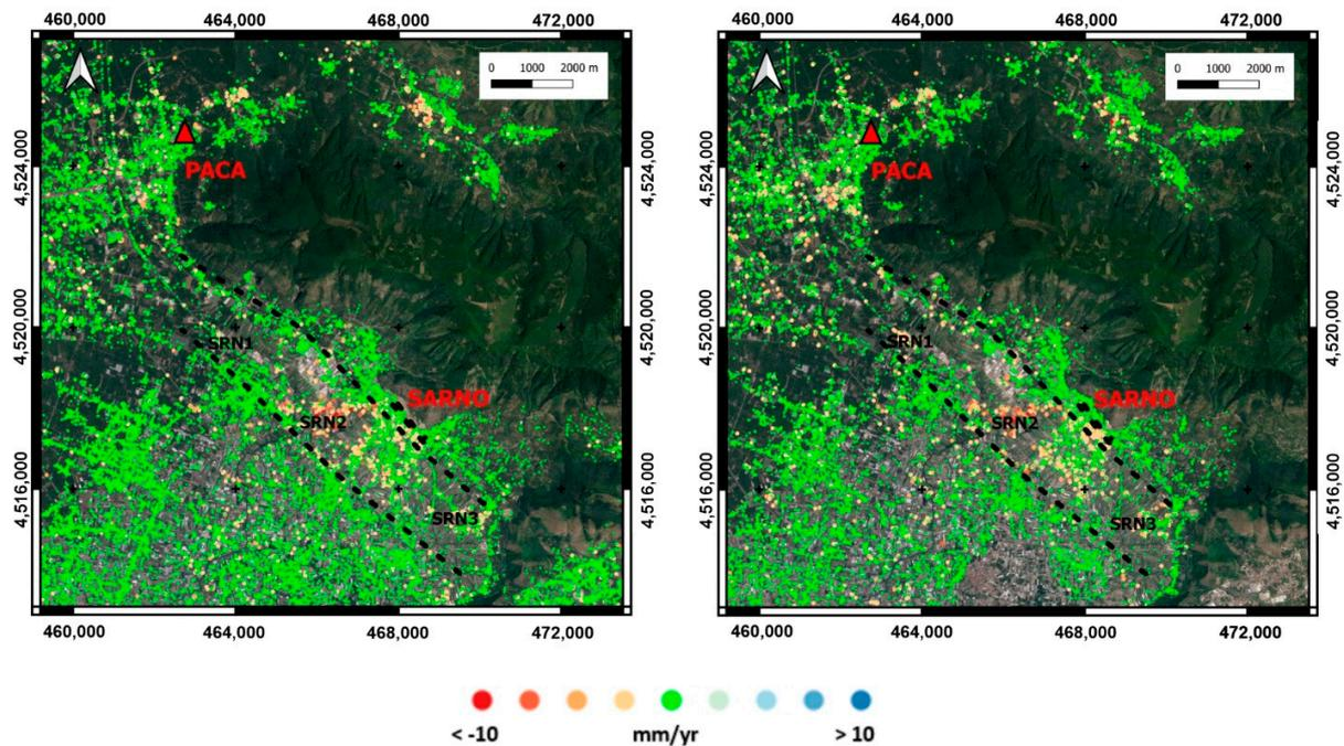
**Figure 11.** Mean displacement rate map for ENVISAT images (2003–2010 period): (a) ascending and (b) descending. Red triangle indicates location of GNSS Palma Campania (PACA).
