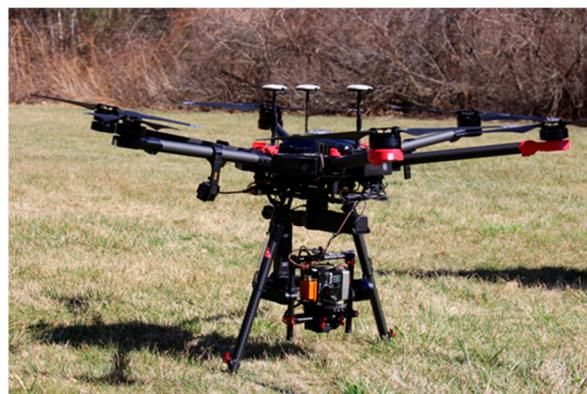
**Figure 2.** Photograph of UAV hyperspectral imaging system.
