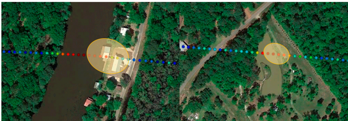
Figure 5. Blowup of the pond (right) and river (left) crossings from Figure 3, with yellow ellipses indicating the approximate orientation and size of the surface spot size, as derived from their respective power measurements vs time.
