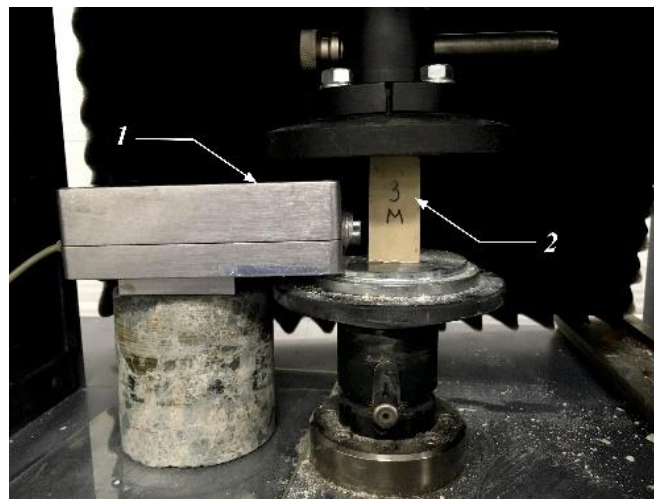
Figure 8. Experimental setup: IR radiation detector (1) and limestone sample (2).
