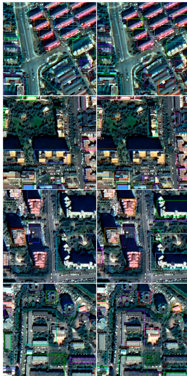
Figure 7. Prediction results of the model on the test set. The four rows show the results on different regions. The left column shows the prediction of mode B, and the right column shows the “TP”, “FP”,
