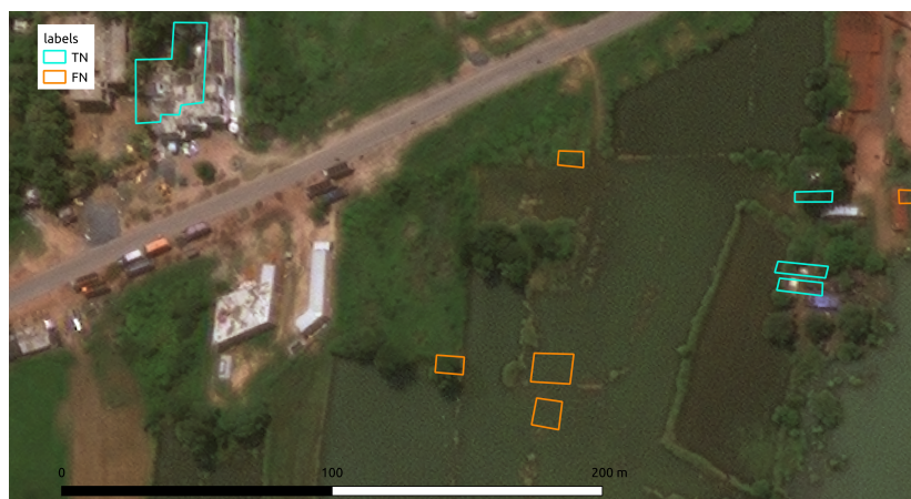
Figure 18. The predictions, true negatives (TN), and false negatives (FN) on 9 out of the 29,808 buildings of the Nepal flooding by the model trained on the Midwest flooding.
