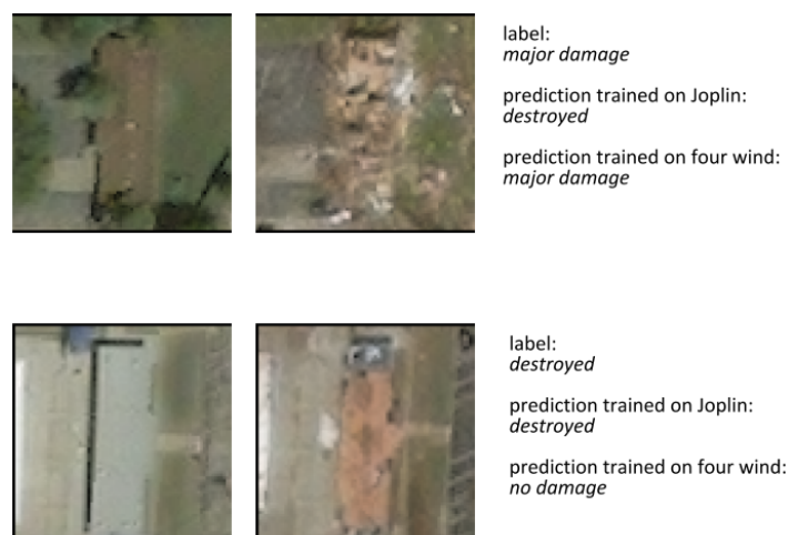
Figure 14. Two buildings before and after the Joplin tornado, and the predictions made by the model trained on the Joplin tornado and the model trained on the four wind disasters .
