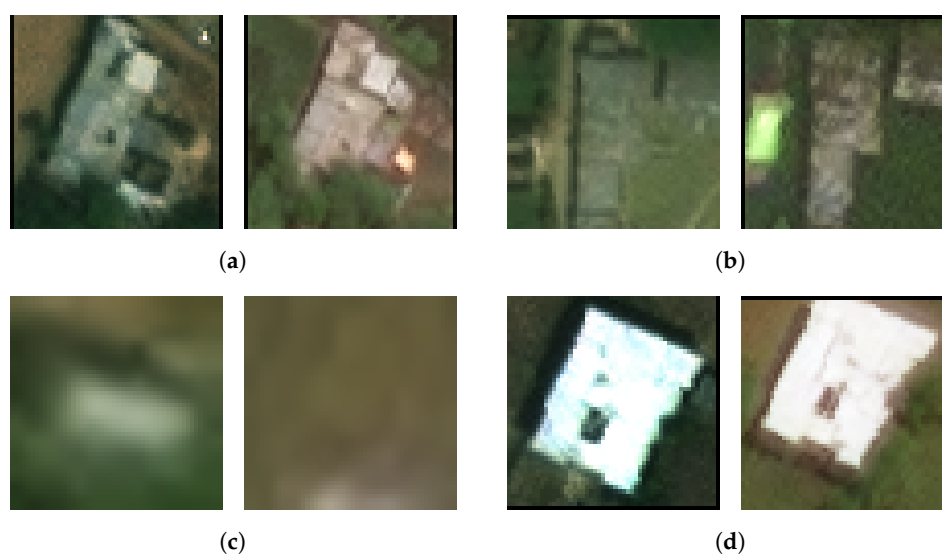
Figure 7. Four examples of buildings in the test set of the Nepal flooding that were misclassified by the model. For each building, the before image is shown on the left and the after image on the right. (a) Label: major damage; prediction: no damage; (b) Label: major damage; prediction: no damage; (c) Label: no damage; prediction: destroyed; (d) Label: no damage; prediction: major damage.
