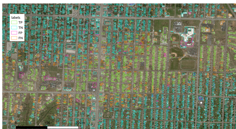
Figure 15. The true positive (TP), true negative (TN), false positive (FP), and false negative (FN) predictions on 2395 out of 12,165 buildings of the Joplin tornado by the model trained on a mixture of four disasters with wind damage.
