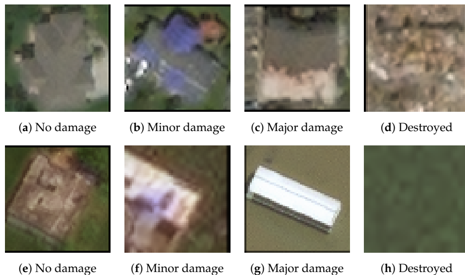
Figure 5. Examples of individual buildings after the disaster impacted by the Joplin tornado ( a–d ) and the Nepal flooding ( e–h ). The subcaptions indicate the damage class.
