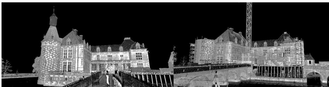
**Figure 3.** TLS intensity-based rendering of the point cloud of the castle acquired before the renovation in February 2016 (left image), and in April 2019 during the renovation (right image).
