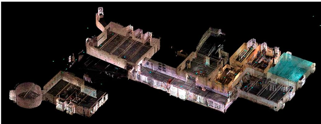
**Figure 13.** Point cloud of the first floor of the castle of Jehay, before the renovations.
