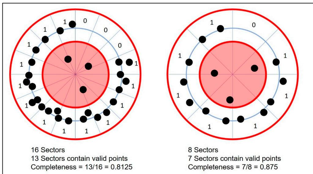
**Figure A2.** An example of how Circumferential Completeness Index (CCI) can be applied to lower-resolution point clouds using fewer sector divisions with a trade-off in precision. Even with reduced precision, CCI can still provide a comparable measure of circumferential coverage of a stem, provided that there is sufficient resolution to fit a circle to the stem slice.
