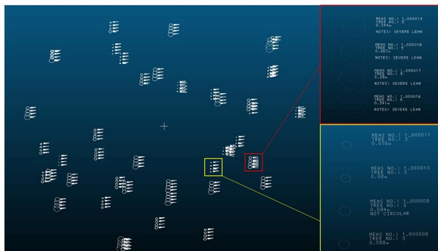
**Figure 4.** Manual field measurements were visualized as a point cloud so that they could be used to correctly identify the corresponding point cloud slice for each measurement. Field notes such as “Severe lean” and “Not circular” were also shown in the visualization to minimize the risk of incorrectly matching a manual measurement with its corresponding point cloud slice.
