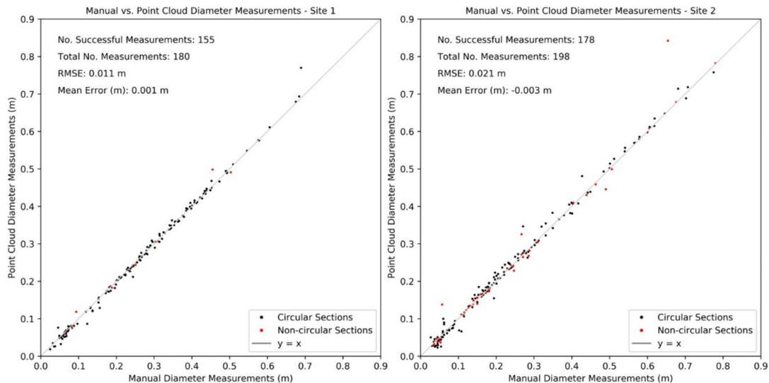
**Figure 10.** Scatter plots of manual diameter measurements obtained in the field using measuring tape- versus the point cloud-based diameter measurements for Site 1 (Left) and Site 2 (Right). Any measurements marked with the qualitative label of “noncircular” are shown as red points and would be expected to have greater error than the circular measurements.
