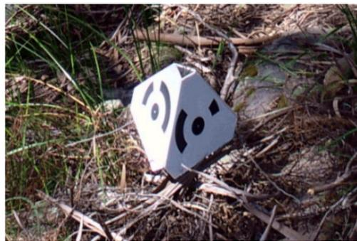
**Figure 6.** Tetrahedron-shaped coded target markers can be quickly deployed in the field to assist the image alignment process. Such coded targets can be automatically detected in Agisoft Metashape and are treated as true matches in the alignment process.
