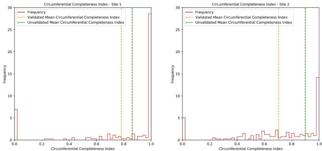
**Figure 13.** Histograms showing Circumferential Completeness Index (CCI) for Site 1 (Left) and Site 2 (Right). Measurements with a completeness score of 0 are measurements which were not sufficiently well captured in the point cloud to extract a clear stem circle. Measurements with CCI of 1 were those with a fully reconstructed stem circle.
