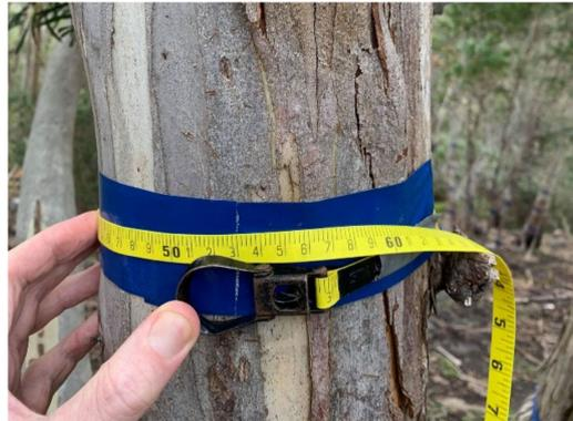
**Figure 5.** Manual field measurements of stem circumference were collected over blue marking tape such that both manual and photogrammetric point cloud-based measurements could be taken from the same location on the tree without influence of a digital terrain model.
