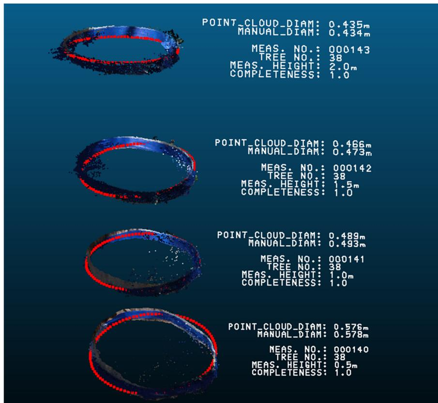
**Figure 8.** Visualization of the circles (shown in red) which were fitted using random sample consensus (RANSAC) to the manually sliced blue marking tape stem circles. The measurements shown above are: RANSAC fitted circle diameter (POINT\_CLOUD\_DIAM), manually measured diameter (MANUAL\_DIAM), and Circumferential Completeness Index (COMPLETENESS).
