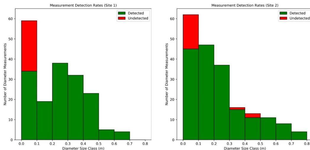
**Figure 14.** Histograms showing detection rates for Site 1 (Left) and Site 2 (Right). The undetected diameter measurements are stacked above the detected diameter measurements to give the total number of measurements in each size class. A stem was considered detected if validated CCI was non-zero.
