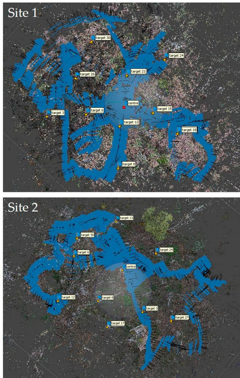
**Figure A1.** Above shows the locations of the 10 tetrahedron-shaped markers placed throughout each site as well as the locations of each image visualized in Agisoft Metashape. These coded targets were placed to assist the image alignment process by providing “true” matches to the solver.
