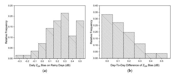
**Figure 15.** (a) Distribution of the daily  $Z_{DR}$  bias of NUIST-CDP. (b) Distribution of the day-to-day difference in the  $Z_{DR}$  bias. The results show that 32% of the day-to-day difference exceeded 0.2 dB, meaning that continuous calibration is highly necessary for NUIST-CDP.
