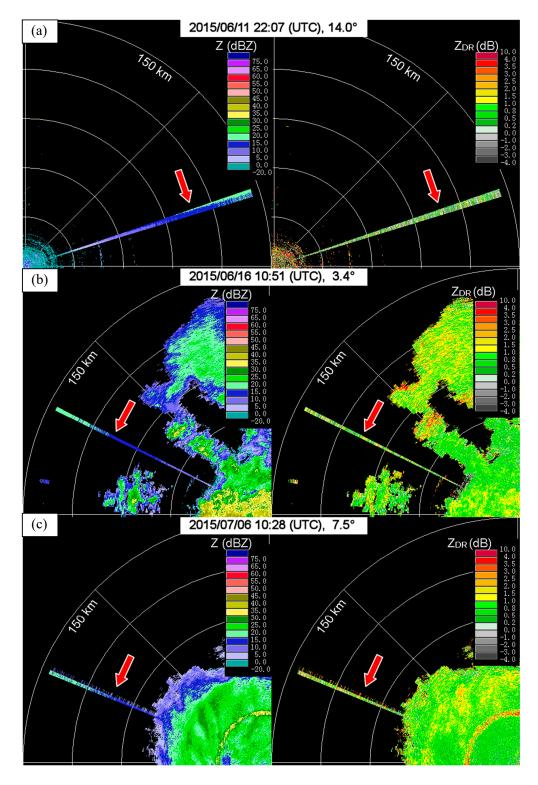
**Figure 3.** Three cases of online solar echoes. (a) Under a clear sky; (b) under weak convective precipitation; (c) under stratiform precipitation. Online solar radials are indicated by red arrows. Clearly, online solar echoes do not only appear under clear sky conditions but sometimes coexist with weak precipitation.
