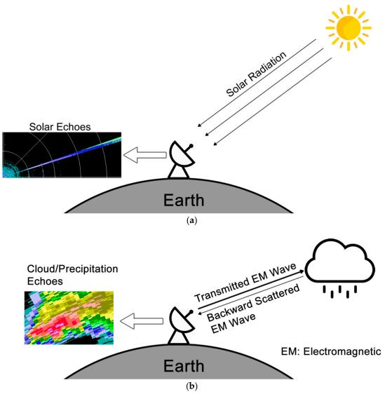
Figure 1. Conceptual sketches of radar echoes from the sun (a) and from cloud/precipitation (b).
