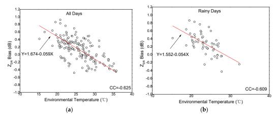
**Figure 13.** The observed relationship between daily  $Z_{DR}$  bias and ambient temperature from June to August 2015. (a) Data for all days. (b) Data on the rainy days. The results show that the  $Z_{DR}$  bias of NUIST-CDP was significantly correlated with the ambient temperature, with a correlation coefficient of about –0.6.
