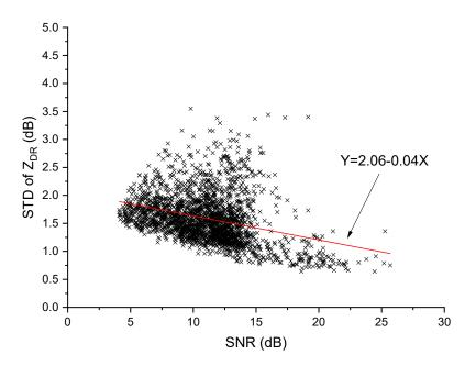
**Figure 6.** The relationship between the signal to noise ratio (SNR) and the standard deviation of  $Z_{DR}$ . Thus, the variance caused by noise should be considered in the estimation of the solar  $Z_{DR}$ .
