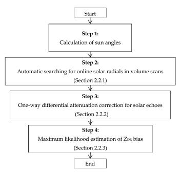
Figure 2. Flow chart of the proposed automatic calibration method based on online solar echoes.
