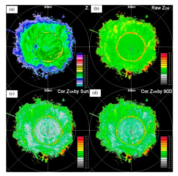
**Figure 12.** Plan position indicator (PPI) images of a case observed at 10:28 UTC on 06 July 2015 at the elevation angle of 7.5°. (a) Observed reflectivity factor. (b) Observed  $Z_{DR}$ . (c) Corrected  $Z_{DR}$  by the proposed online solar method. (d) Corrected  $Z_{DR}$  by the vertical pointing method. Clearly, the corrected  $Z_{DR}$  by the proposed online solar method is closer to that corrected by the vertical pointing method (truth) than the uncorrected  $Z_{DR}$ .
