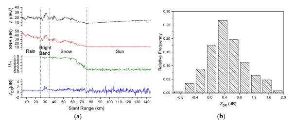
**Figure 5.** Distribution of online solar echoes along the radial direction. (a) Range profiles. The characteristics of solar echoes were largely different from those of meteorological echoes. (b) The histogram of solar  $Z_{DR}$ . Clearly, the probability density function of solar  $Z_{DR}$  shows an approximately Gaussian distribution, which means that the method in Section 2.2.3 could be used to obtain the optimal estimation.
