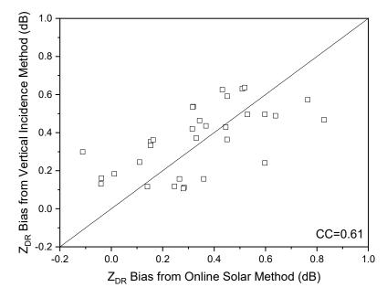
**Figure 8.** The daily  $Z_{DR}$  bias of the online solar method and the vertical pointing method. The results show that the results of the proposed method were correlated with those of the traditional vertical pointing method.
