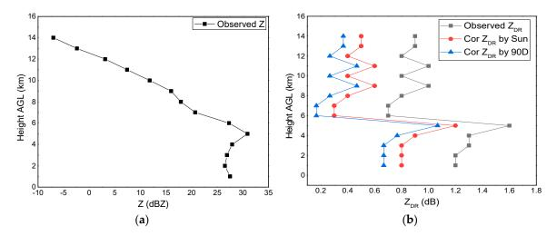
**Figure 11.** (a) Vertical profile of Figure 10a. (b) Vertical profiles of Figure 10b–d. The results suggest that the corrected  $Z_{DR}$  by the proposed online solar method was reasonable and closer to that corrected by the vertical pointing method (truth) than the uncorrected  $Z_{DR}$ .
