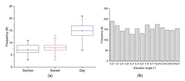
**Figure 4.** Frequency of occurrence of online solar echoes in the volume scan. (a) Boxplot and (b) frequency distribution with elevation angle. Clearly, online solar echoes occurred very frequently and appeared at a similar frequency at each elevation angle. This characteristic was favorable for the monitoring of daily differential reflectivity ( $Z_{DR}$ ) bias.
