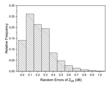
**Figure 14.** Distribution of the random error of Z<sub>DR</sub> from NUIST-CDP based on an analysis of a case of uniform snowfall.
