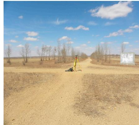
**Figure 5.** Experimental data and reference data at the Taihang research area. (a) Spatial coverage of the research area; (b) image showing a GCP (Ground Control Point) measured primarily by using a static Global Positioning (GPS) receiver.
