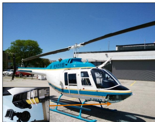
Figure 2. Hyperspectral sensor mounted on a helicopter.
