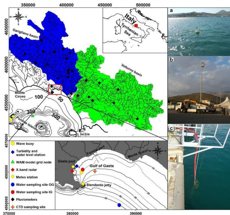
**Figure 1.** Regional view of the study area with a detail of the Gulf of Gaeta (red rectangle) and the localization of devices installed in the study area. (a) Wave buoy in the Gulf of Gaeta; (b) X-band radar installed on the lighting pole; (c) Turbidity station installed on the dock.
