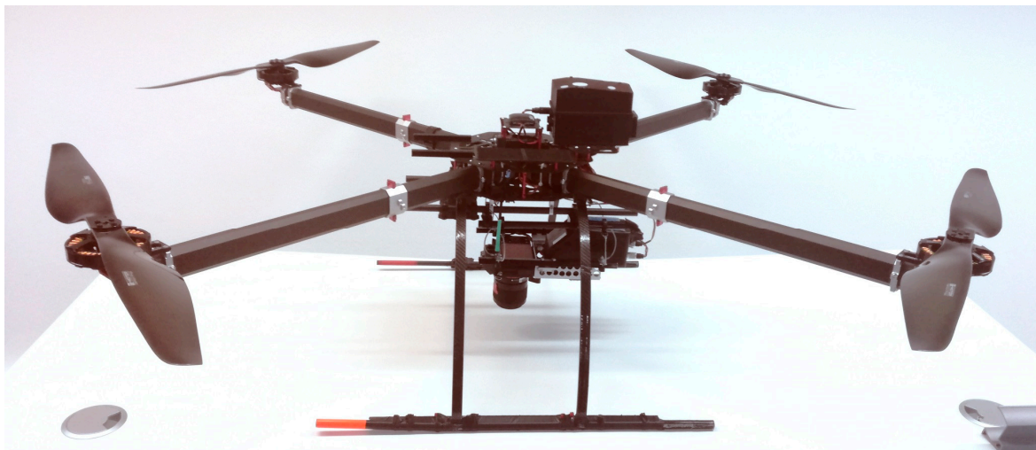
Figure 3. The unmanned aerial vehicle (UAV) set-up used in the mapping experiment. The FGI AIRS is installed on top of the UAV, while the FPI2012b hyperspectral camera and the Sony A7R consumer camera are installed under it.
