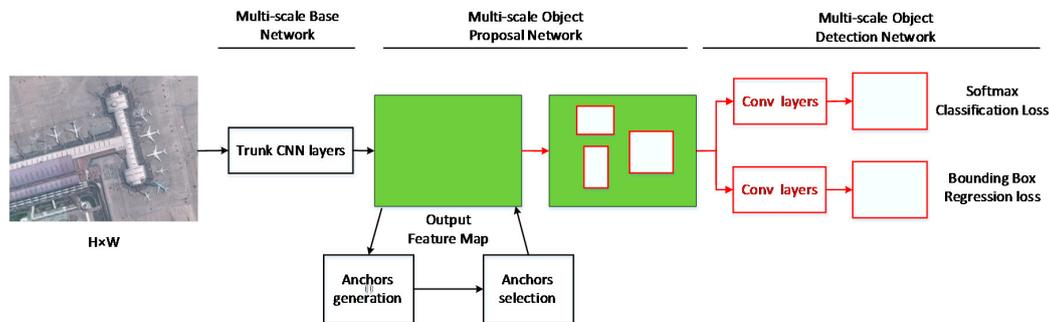
**Figure 2.** Architecture of the unified multi-scale CNN.
