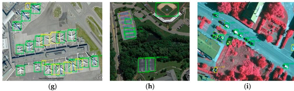
**Figure 6.** Detection results using our method, Faster R-CNN and SSD. The first row are results of our method; the second row are results of Faster R-CNN; the third row are results of SSD.
