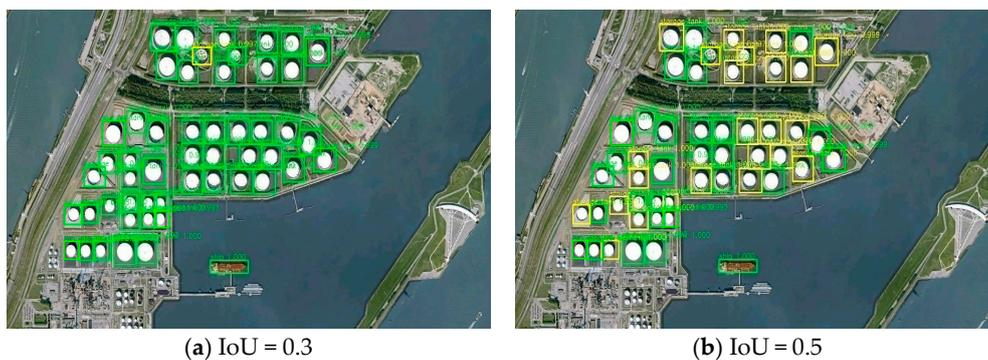
**Figure 10.** Detection results of storage tanks under different IoU.
