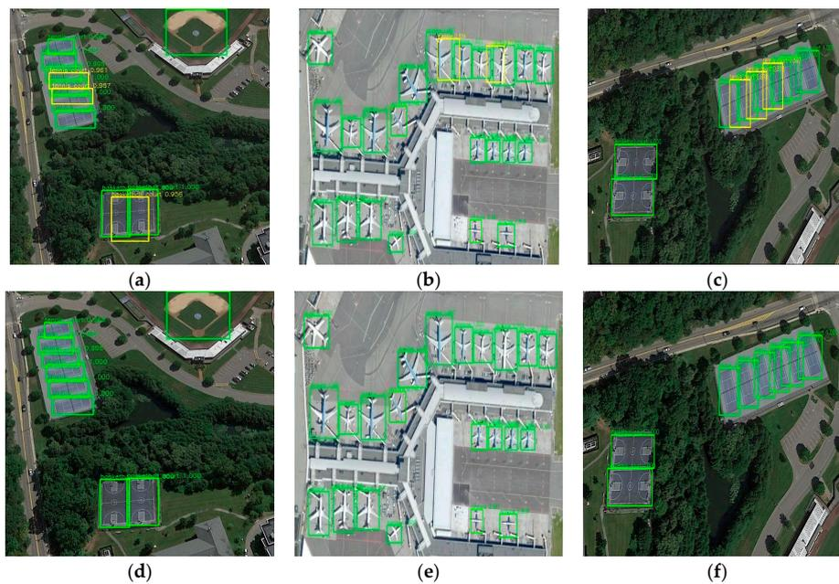
**Figure 8.** Detection results using our method with NMS and Soft NMS. The first row are results of our method with NMS; the second row are results of our method with Soft NMS.
