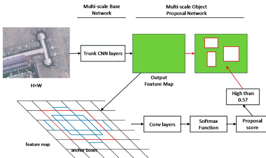
Figure 5. Architecture of the multi-scale object proposal network.
