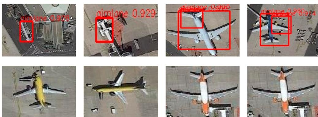
Figure 12. Some typical false alarms and missing targets among the detection results of our method: the first row are some typical false alarms, while the second row are some missing targets.
