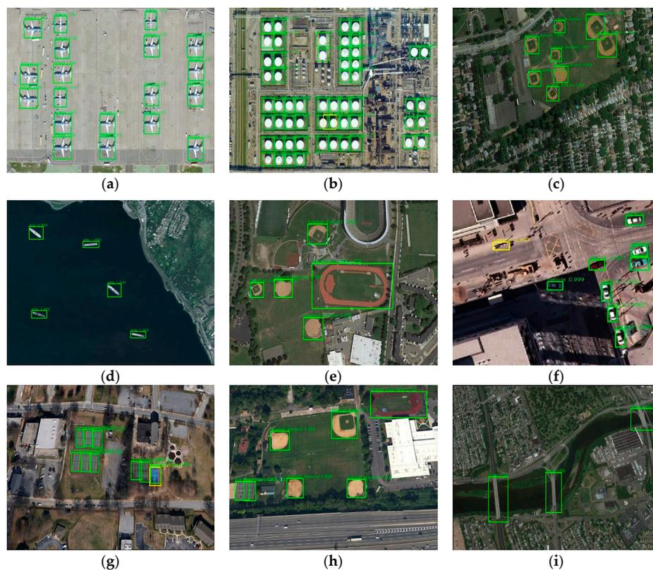
**Figure 7.** Detection results using our method.
