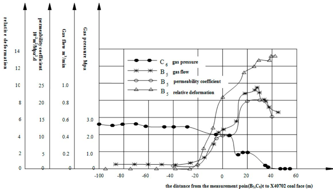
Figure 8. Variations in the gas parameters of seam 11<sup>#</sup> during UPS mining.
