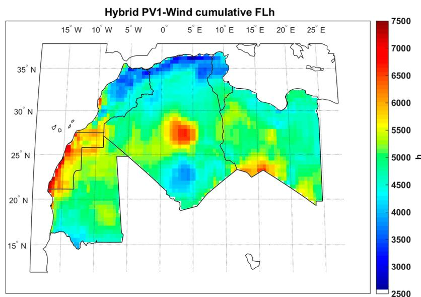
**Figure 4.** Maghreb's hybrid PV–Wind power plant cumulative FLh map.
