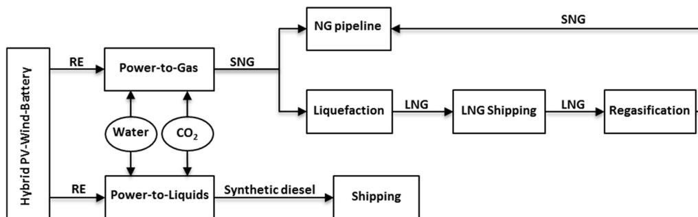
Figure 1. The hybrid PV–Wind-(PtG, PtG–LNG, and PtL) value chain (very simplified).
