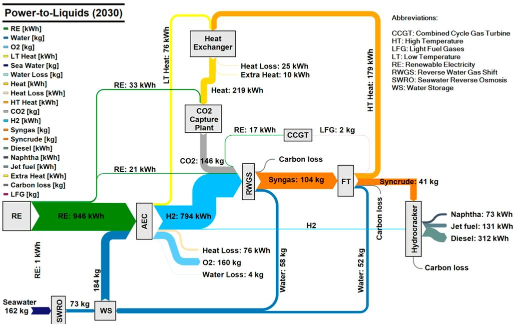
Figure 6. RE-PtL energy and material flow diagram.
