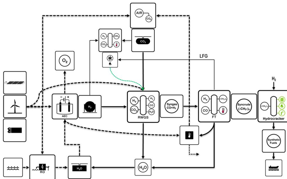
Figure 3. The hybrid PV-Wind-PtL value chain.
