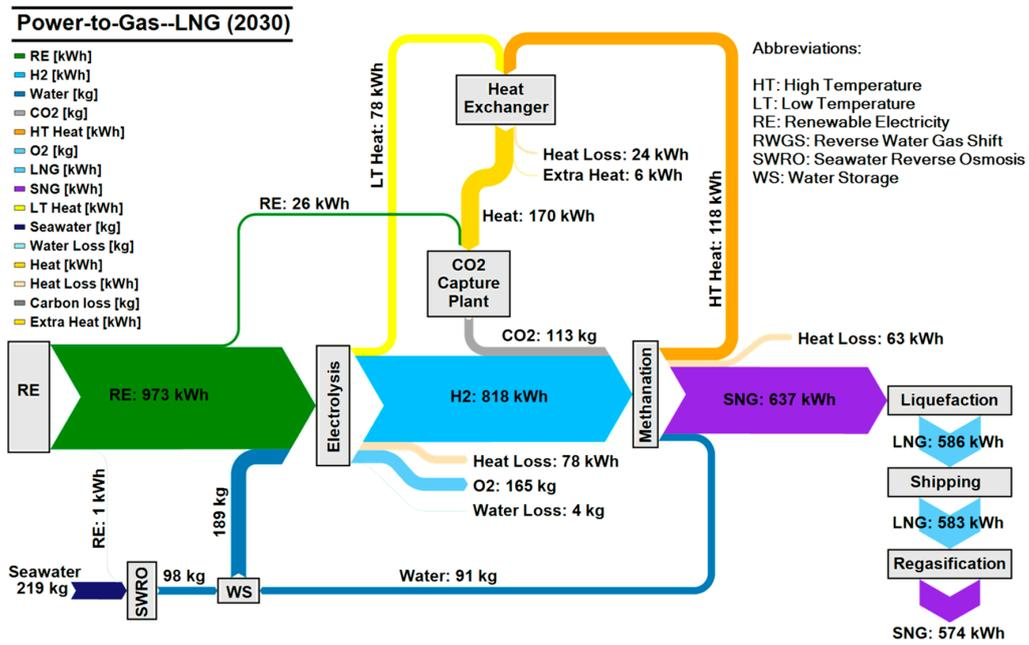
Figure 5. RE-PtG–LNG energy and material flow diagram.
