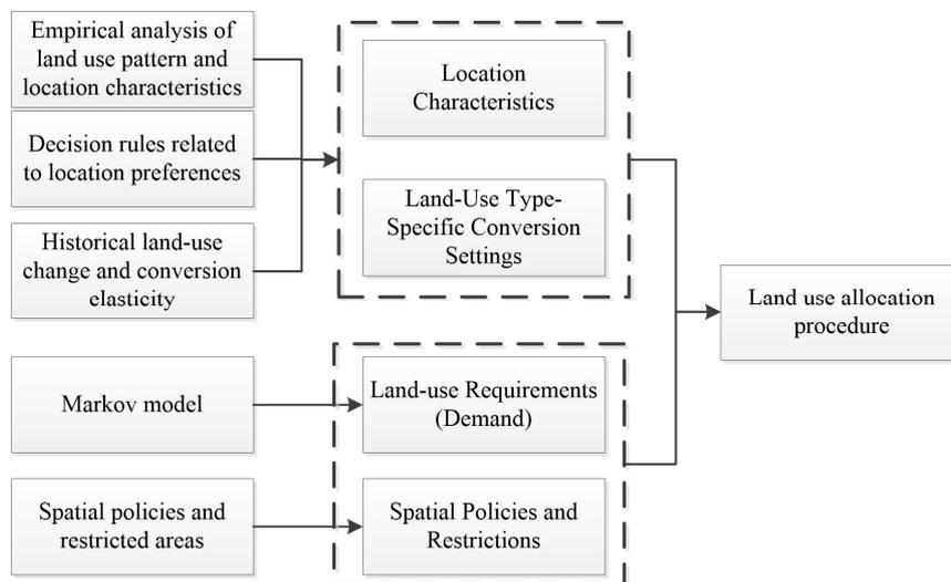
Figure 3. Overview of the information flow in the CLUE-s model used for the study area. Note: This figure is redrawn according to Reference [29].
