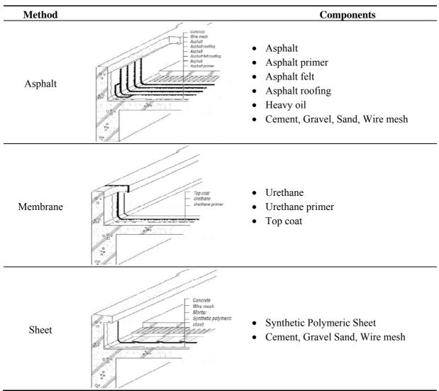
Table 1. Components of roof waterproofing system.
