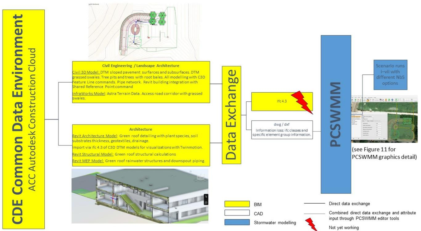
**Figure 4.** BIM/PCSWMM workflow. In this study, certain specific NbS attributes (e.g., hydraulic conductivity) from the BIM design were entered manually in the PCSWMM pull-down dialogue tools such as the LID editor.
