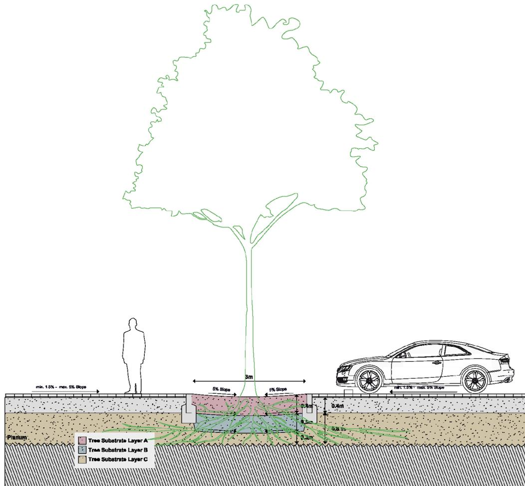
**Figure 7.** The sloped tree substrate system for tree pits in the city of Zürich, which provides more tree root space.
