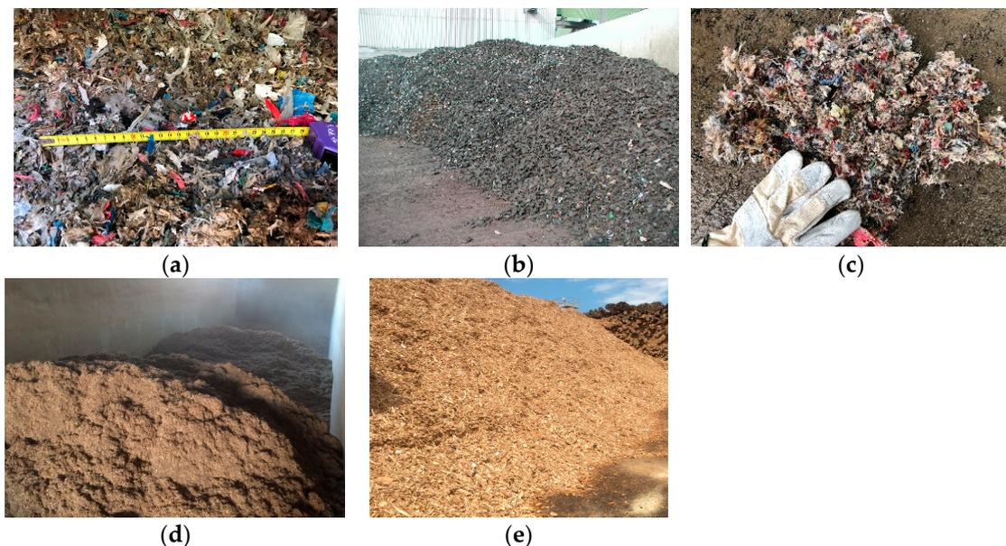
**Figure 2.** Typical AFR resources used as a heat source, e.g., in the cement industry: (a) plastic waste, (b) rubber pieces (e.g., from shredded tires), (c) carpet and cloth waste, (d) biomass, (e) wood chips.
