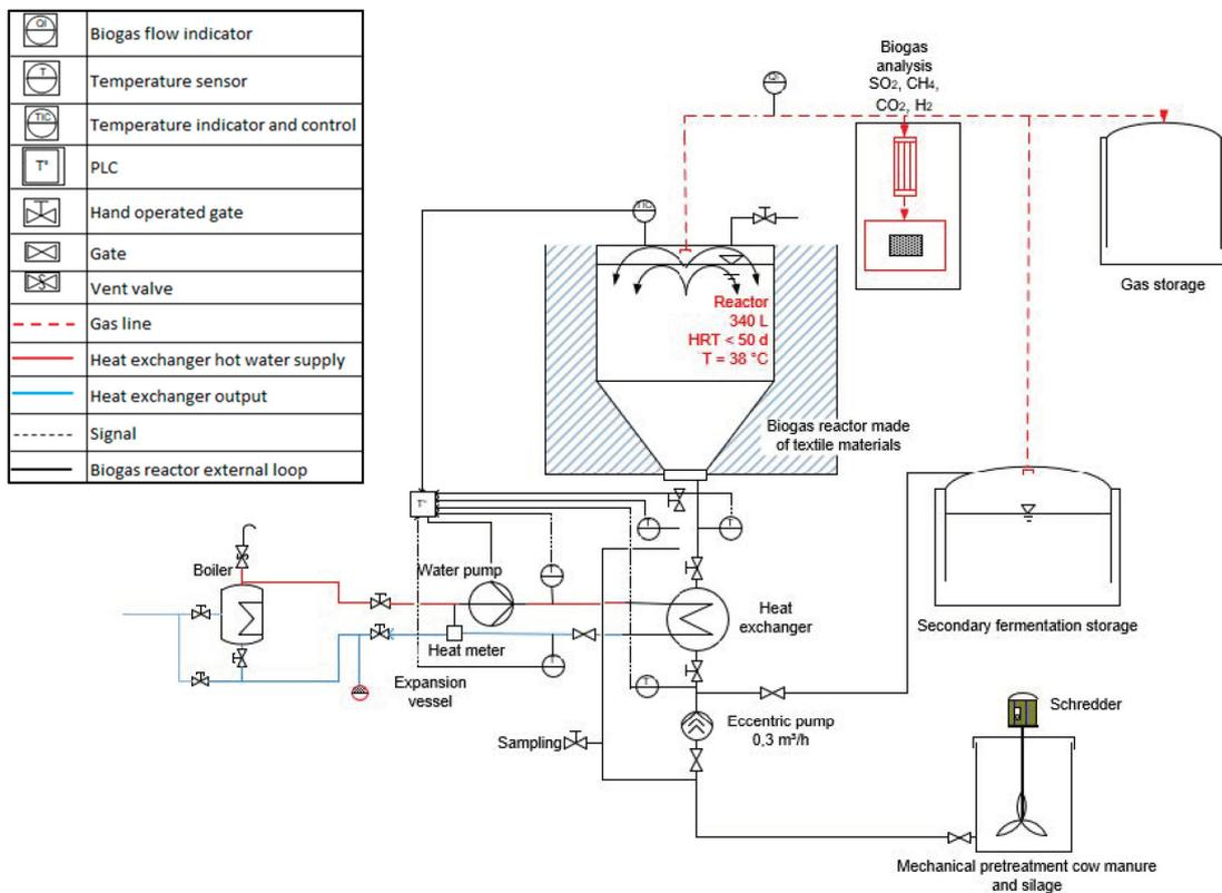
**Figure 2.** Pilot-scale biogas plant flow diagram.
