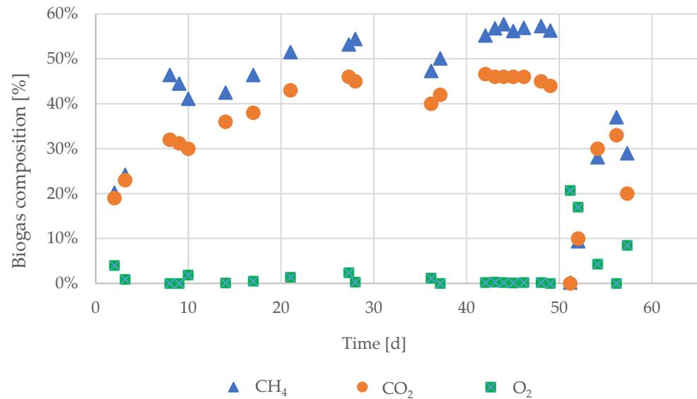
**Figure 7.** Biogas composition during normal operation. The oxygen was introduced during the feeding of the system. The feeding operation occurs by opening and closing the installed ball valve of the pretreatment unit by hand in combination with the eccentric pump suction. If the loading liquid level in the pretreatment vessel decreases enough, air flows into the system.
