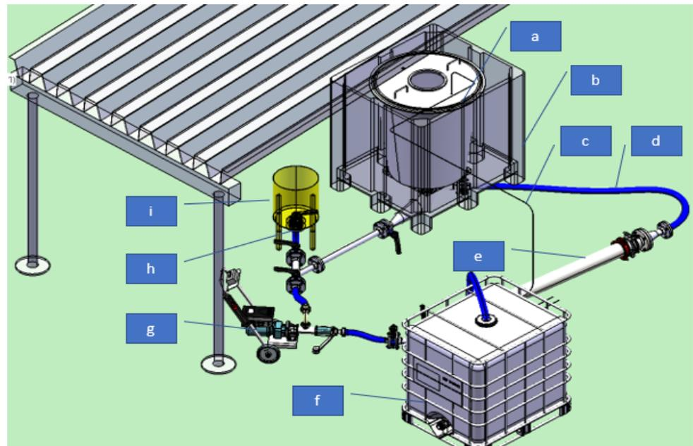
**Figure 1.** 3D representation with (a) biogas reactor, (b) biogas reactor container, (c) gas connection between the biogas reactor and the gas-tight digestate storage, (d) exterior biogas cycle hose, (e) heat exchanger, (f) gas-tight digestate storage, (g) eccentric pump, (h) sand trap and (i) shredding pretreatment unit.
