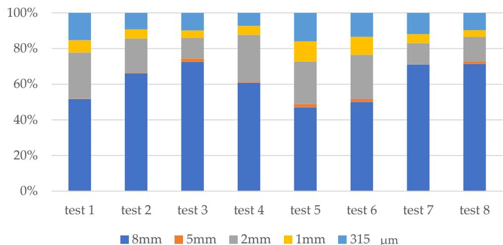
**Figure 4.** Particle size distribution from sieve analysis results. The AS 200 control has 5 sieves with mesh sizes of 8 mm, 5 mm, 2 mm, 1 mm and 315 µm.
