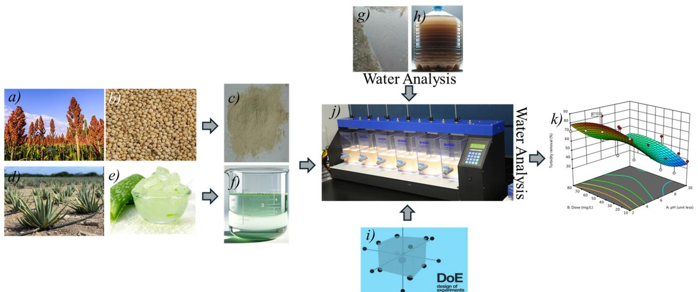
**Figure 1.** Experimental workflow diagram. Stages: (a) Sorghum plant illustration, (b) display of sorghum seeds, (c) ground sorghum seed sample, (d) Aloe Vera plant illustration, (e) extracted Aloe Vera pulp, (f) Aloe Vera pulp solution preparation, (g) water canal sampling location, (h) composite water sample collection, (i) experimental design, (j) jar test apparatus setup, (k) data analysis and optimization phase.
