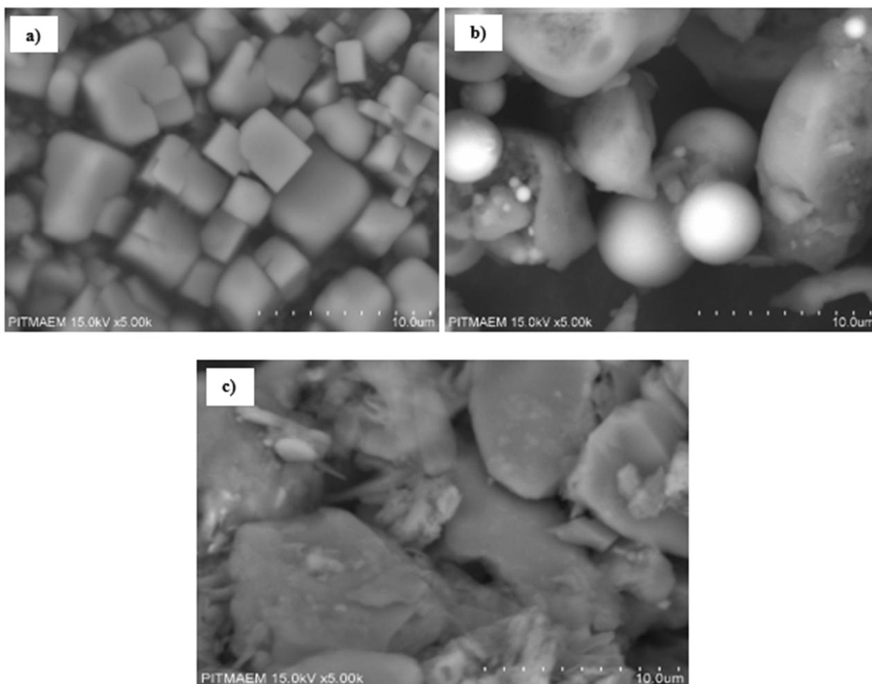
**Figure 11.** SEM images of (a) the Aloe Vera gel, (a) the Sorghum seed powder, (b) the floccs produced after treatment, and (c) Sorghum with Aloe Vera.
