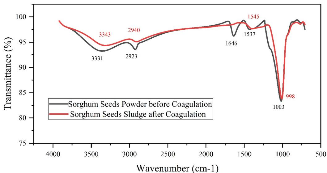
**Figure 5.** FTIR spectra of Sorghum seed powder (black line —) and sludge after treatment (red line —).
