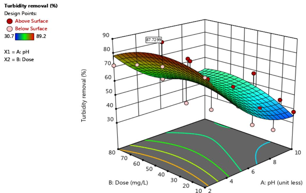
**Figure 2.** 3D response surface plot (Sorghum dose vs. pH) showing the performance (pH = 2; dose = 40 mg/L; turbidity removal = 87.73%; residual turbidity = 38.5 NTU).
