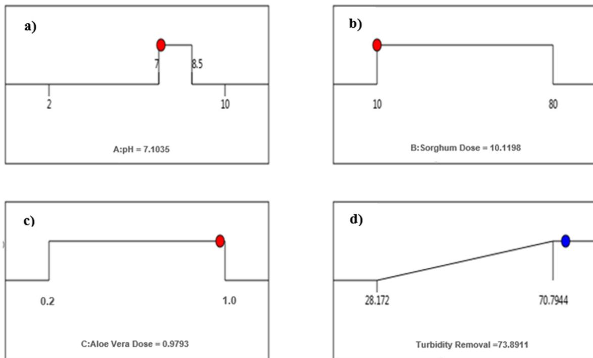
**Figure 10.** Optimization at pH range 7–8.5: (a) pH = 7.1; (b) Sorghum dose = 10.1 mg/L; (c) Aloe Vera dose = 0.98%; (d) turbidity removal = 73.9%. Red balls show the input variables while blue balls show the response value (turbidity removal efficiency).
