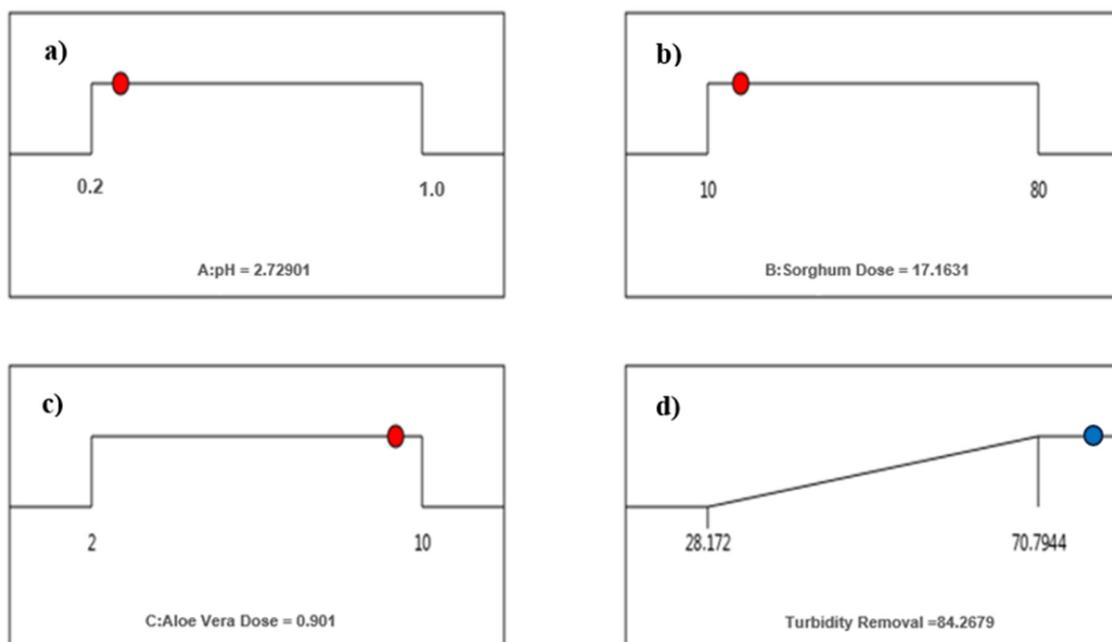
**Figure 9.** Optimization of treatment variables: (a) pH = 2.7; (b) Sorghum dose = 17.1 mg/L; (c) Aloe Vera dose = 0.9%; (d) turbidity removal = 84.2%. Red balls show the optimal input variables while blue balls show the optimal response (turbidity removal efficiency).
