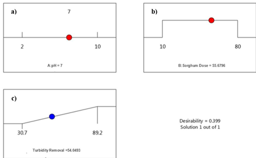
**Figure 4.** Optimization of treatment variables at pH range 7–8.5: (a) pH = 7; (b) dose = 55.7 mg/L; (c) turbidity removal = 54%. Red balls show the input variables while blue balls show the response value (turbidity removal efficiency).
