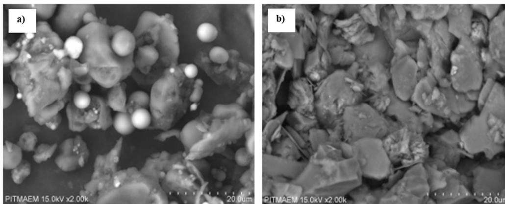
**Figure 7.** SEM images of (a) Sorghum seed powder and (b) flocs produced after treatment.
