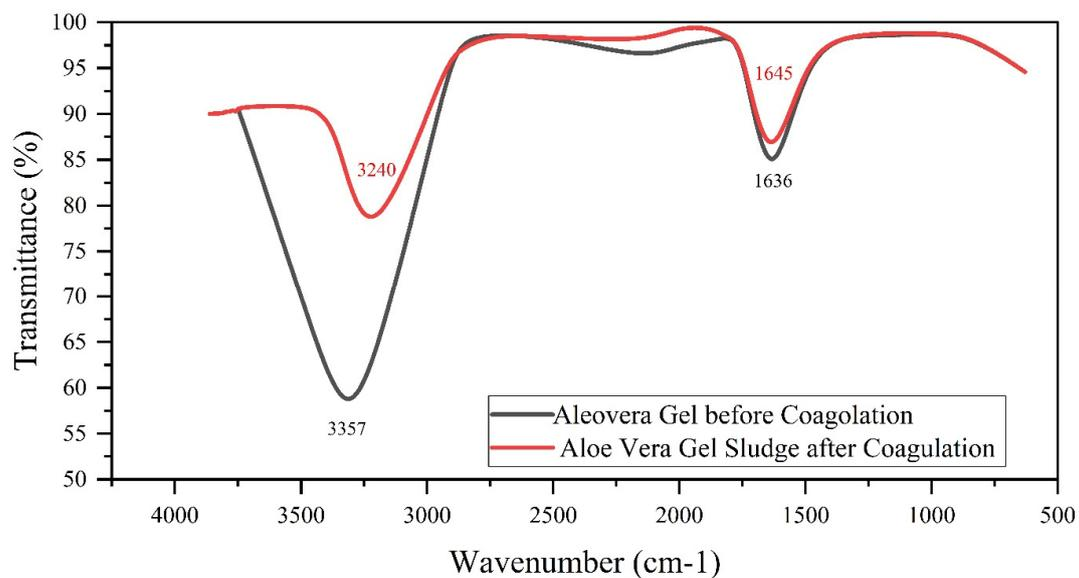
**Figure 6.** FTIR spectra of Aloe Vera gel (black line —) and Aloe Vera gel sludge after treatment (red line —).
