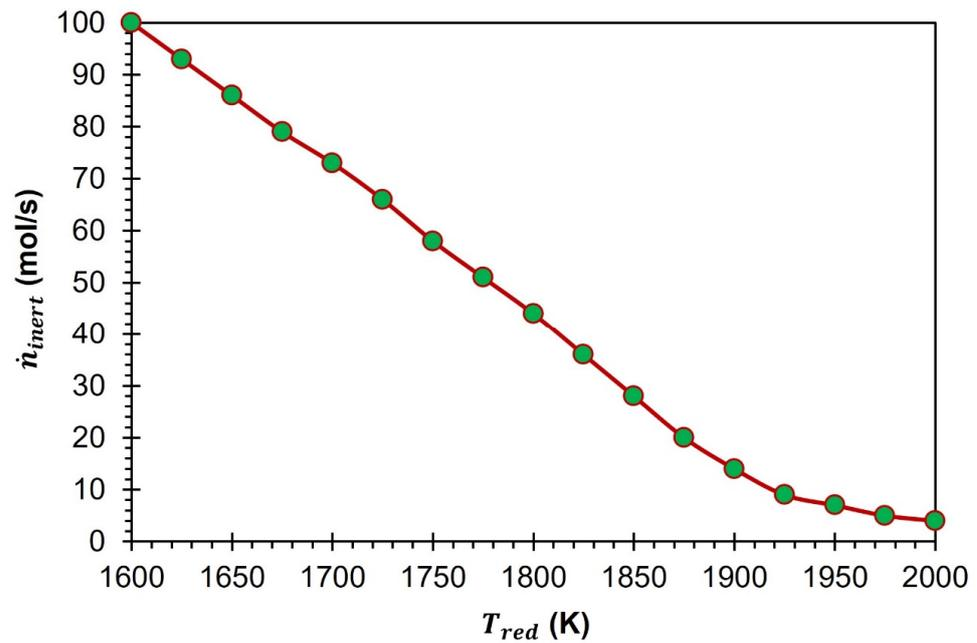
**Figure 2.**  $\dot{n}_{inert}$  needed for the complete reduction of  $\text{GeO}_2$  at  $T_{red}$  in the range of 1600 to 2000 K.
