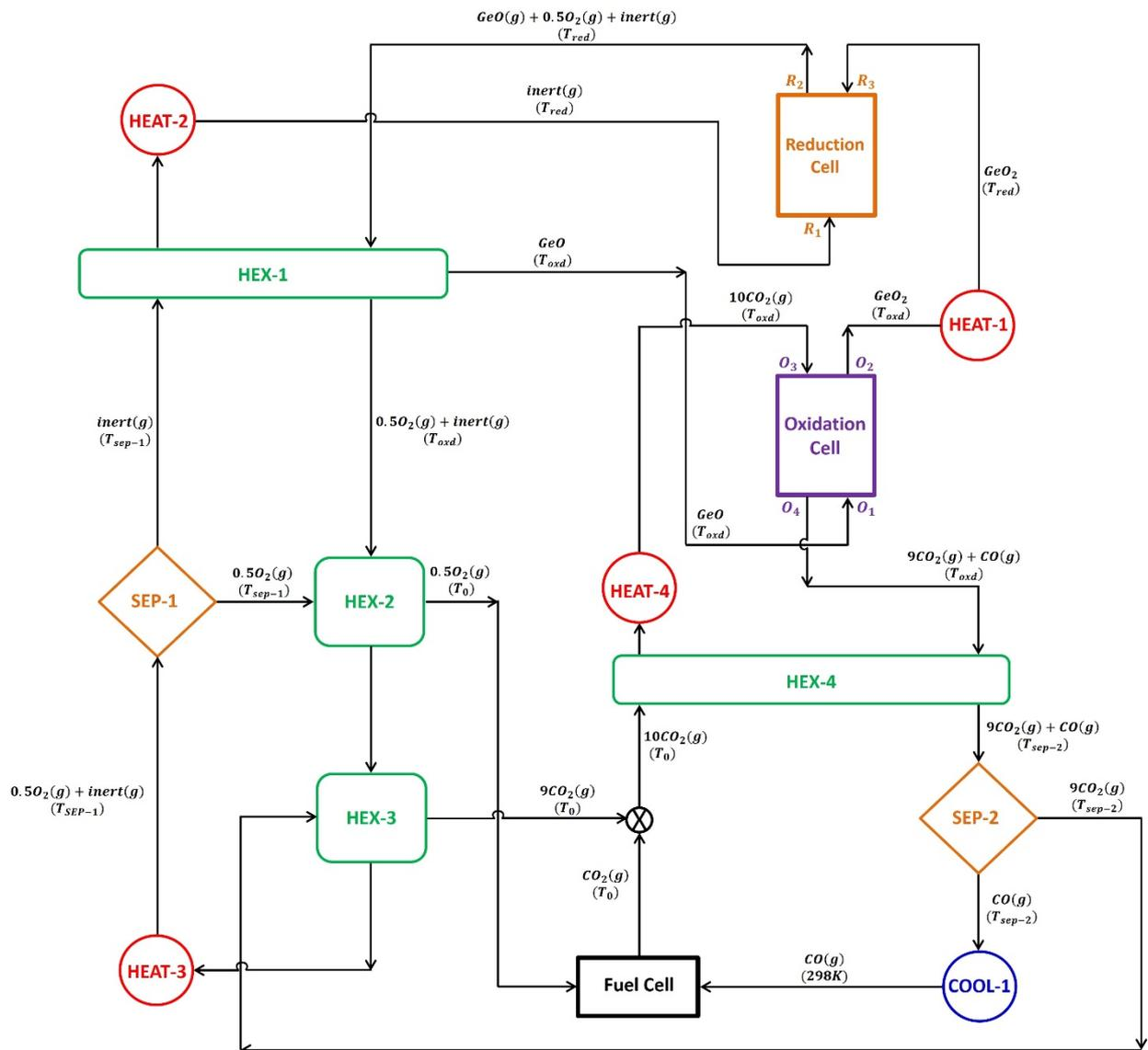
**Figure 1.** A process model of the  $\text{GeO}_2/\text{GeO}$  redox thermochemical cycle for  $\text{CO}_2$  conversion into solar fuels.
