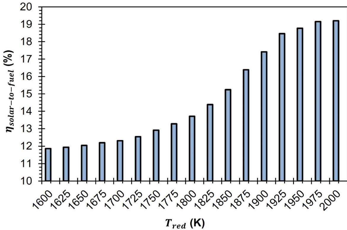
Figure 12. Variation in the  $\eta_{solar-to-fuel}$  of GeO<sub>2</sub>/GeO-based CDS cycle.
