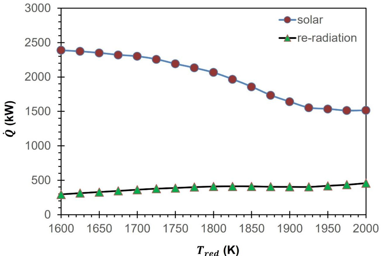
**Figure 11.** Variation in  $\dot{Q}_{solar}$  and  $\dot{Q}_{re-rad}$  for the  $GeO_2/GeO$  CDS cycle.
