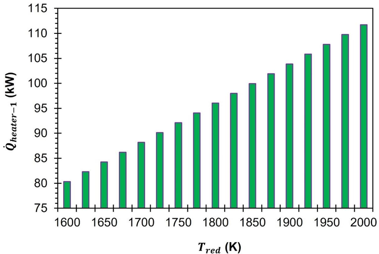
**Figure 5.** Variation in  $\dot{Q}_{heater-1}$  as a function of  $T_{red}$ .
