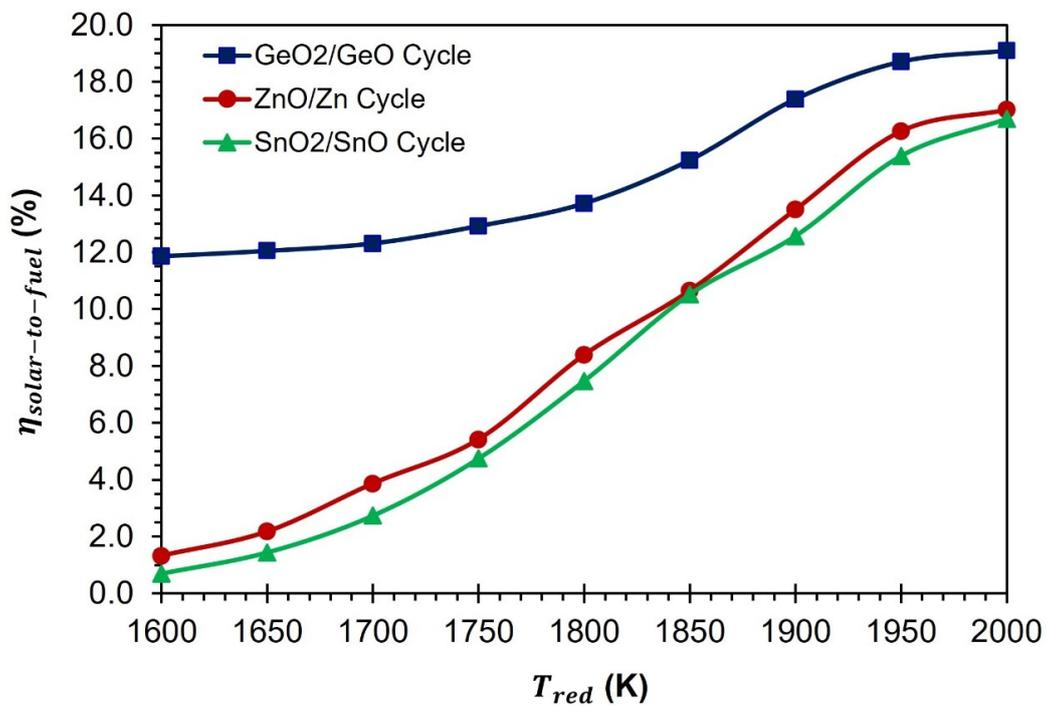
Figure 13. Comparison between the GeO<sub>2</sub>/GeO-based, ZnO/Zn-based, and SnO<sub>2</sub>/SnO-based CDS cycles based on  $\eta_{solar-to-fuel}$ .
