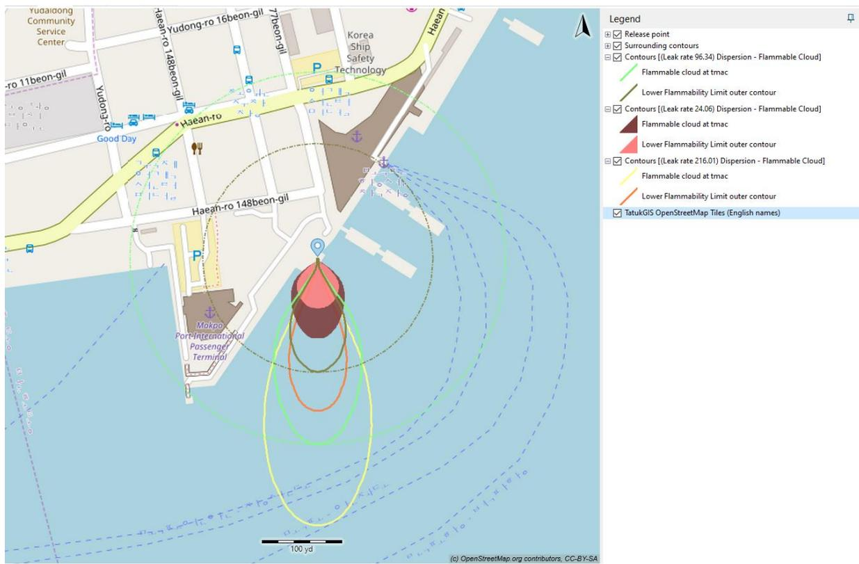
Figure 8. Comparison of vapor cloud dispersion for 3 leak rate values.
