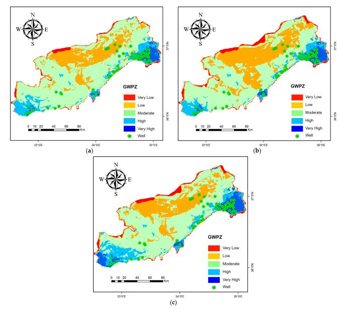
**Figure 7.** (**a**) Groundwater potential maps of the study area obtained by the (**a**) AHP, (**b**) VIKOR, and (**c**) TOPSIS methods.
