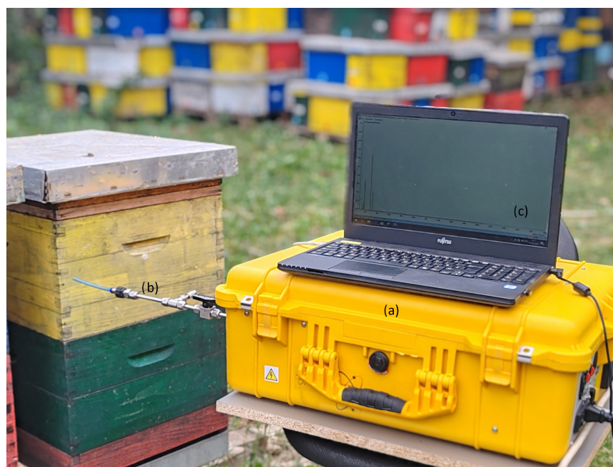
Figure 1. In-field system setup: (a) Portable membrane inlet mass spectrometer with (b) sampling probe and (c) laptop for acquisition and processing of the results.
