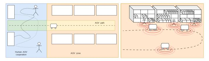
Figure 4. Examples of sharing space between humans and AGVs.
