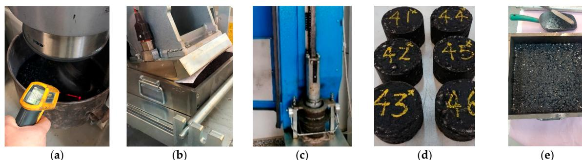
**Figure 5.** Manufacturing procedure and compaction of specimens: (a) mixing; (b) compaction of slabs with the roller compactor; (c) compaction of cylindrical specimens by impact; (d) cylindrical specimens; (e) slabs.
