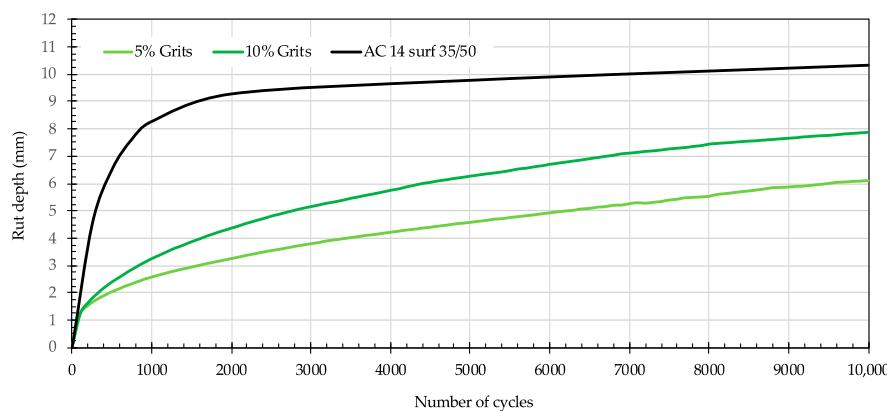
**Figure 11.** Variation of rut depth in wheel-tracking test results.
