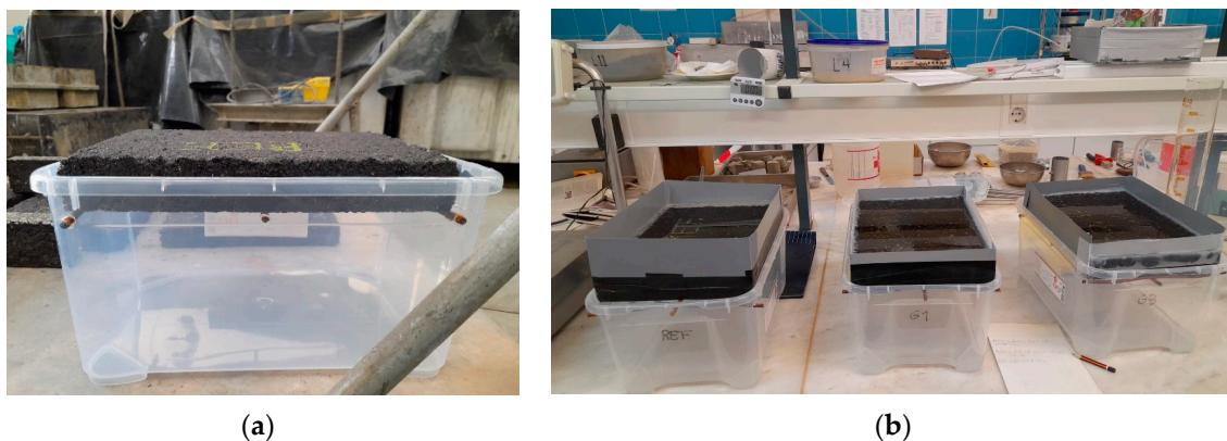
**Figure 7.** Water load test: (a) detail of the supporting box and its slab; (b) testing procedure.
