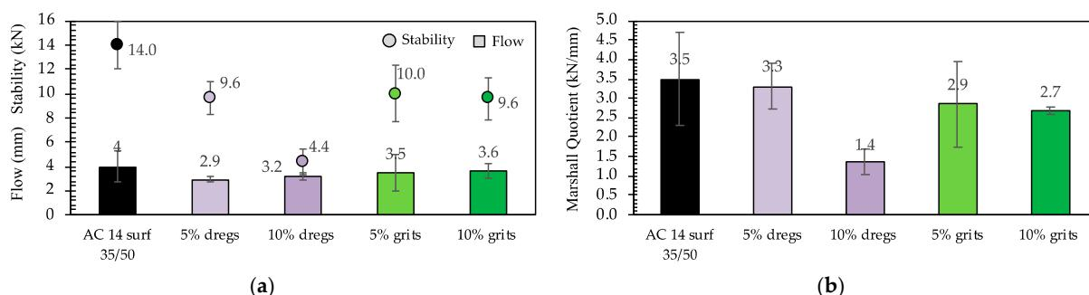
**Figure 10.** Marshall properties: (a) stability and flow; (b) Marshall quotient.
