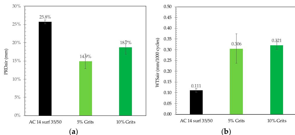
**Figure 12.** Results derived from wheel-tracking curves: (a)  $PRD_{air}$ ; (b)  $WTS_{air}$ .
