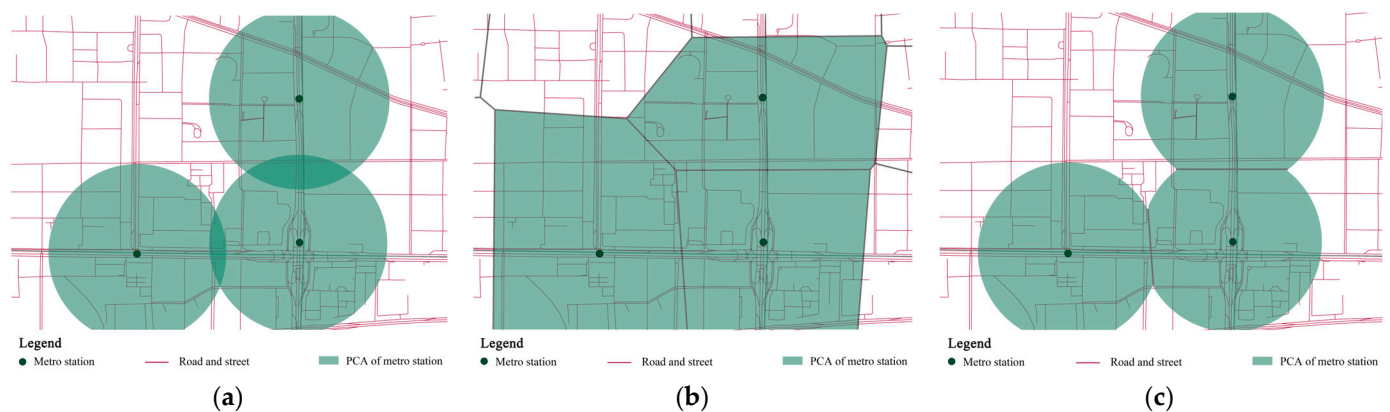
Figure 1. Three PCA delineation methods: (a) circular buffer; (b) Tyson polygon; (c) Tyson polygon superimposed with circular buffer.
