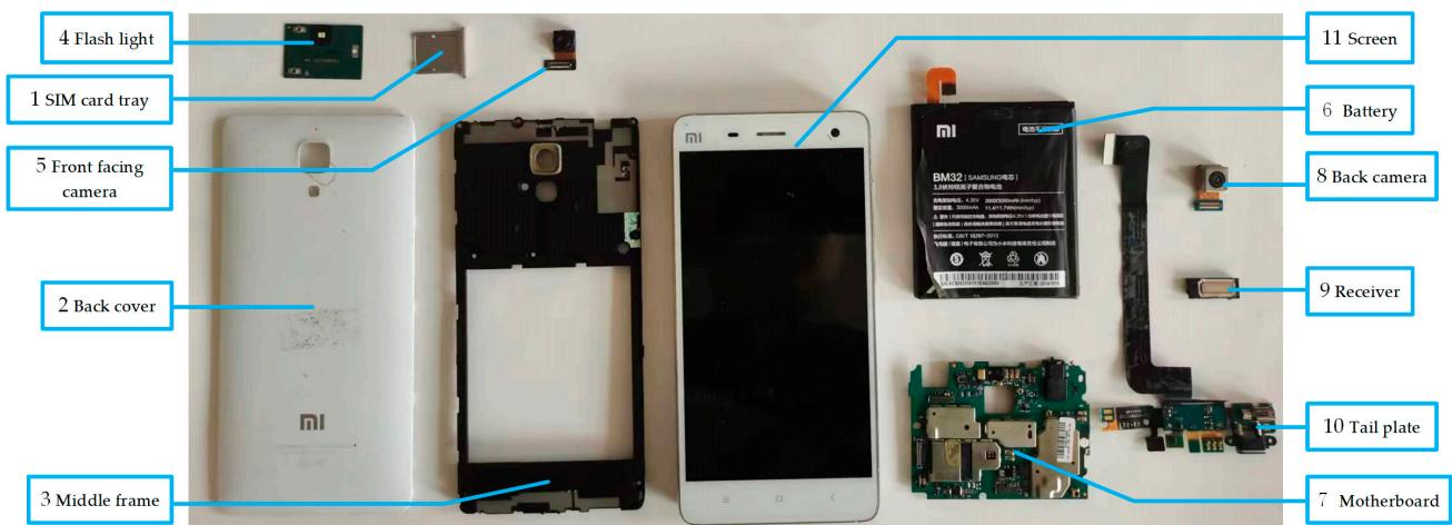
**Figure 7.** The disassembly parts graph for ‘Xiaomi 4’.
