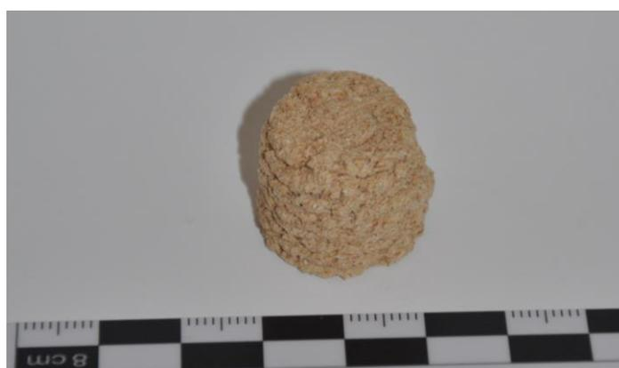
**Figure 5.** Test specimen made of wood dust consisting of spruce and poplar and 15 wt.% alginate.
