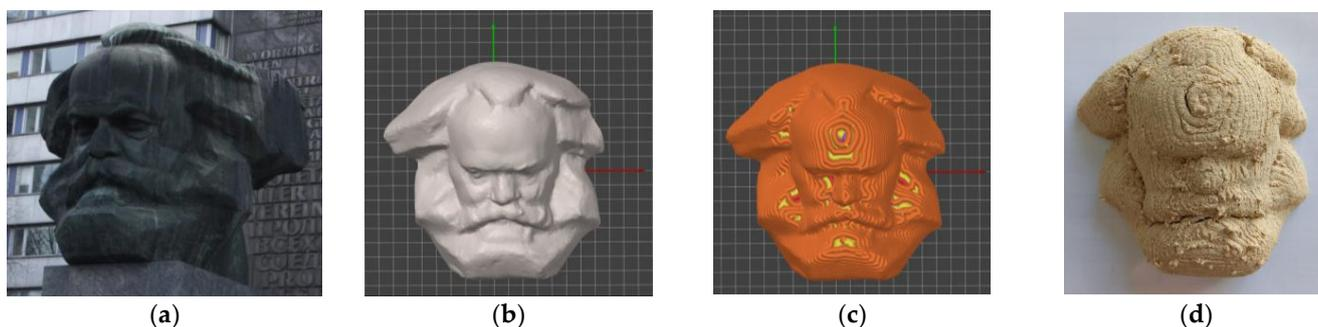
**Figure 6.** Representation of the Karl Marx monument: (a) Original monument; (b) 3D-part of the monument; (c) G-code; (d) Printed part of the monument using the material extrusion process.
