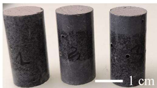
**Figure 1.** Example of cylindrical-shaped grey geopolymer samples based on volcanic ash of Mt. Etna volcano [74].
