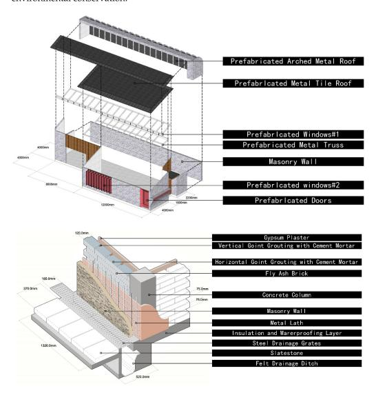
Figure 9. Schematic configuration of semiassembled structure and semiprefabricated buildings.
