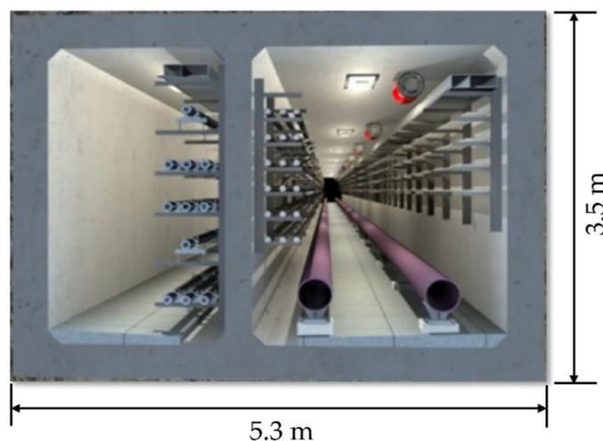
**Figure 3.** Standard internal cross-sectional size of the comprehensive pipe gallery.
