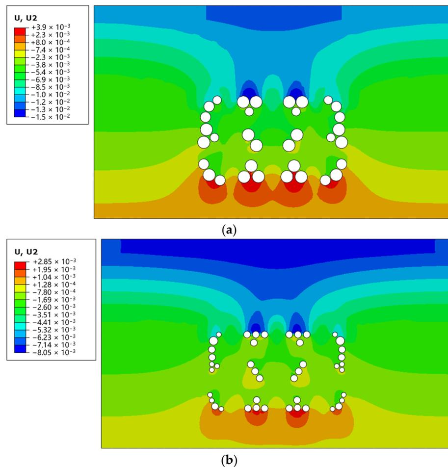
**Figure 7.** Vertical displacement of surrounding rocks (unit: m): (a) case 1; (b) case 2.
