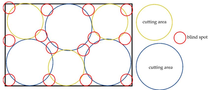
**Figure 1.** Sketch map of blind spots on the working face of a pipe jacking machine with rectangular cross-section.
