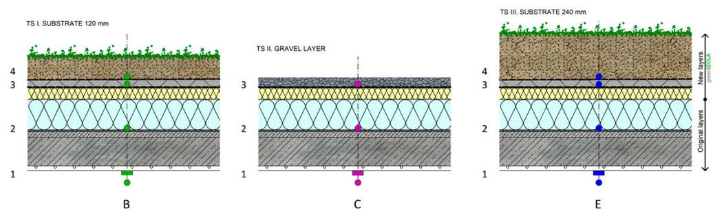
**Figure 6.** Compositions of test segments and placement of sensors in individual layers.
