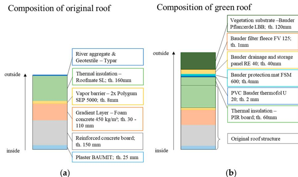
**Figure 4.** Roof composition before (a) and after (b) construction of the green roof of the greenIZOLA building.
