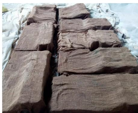
**Figure 6.** The samples covered with wet cloth and nylon.
