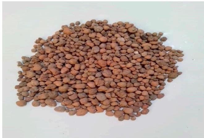
**Figure 1.** LECA coarse grain used in this research as gravel.
