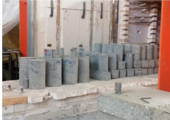
**Figure 7.** The samples prepared inside the furnace.
