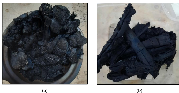
Figure 3. (a) OPP-AC after activation process using KOH (b) OPP-AC after activation using HNO 3 .
